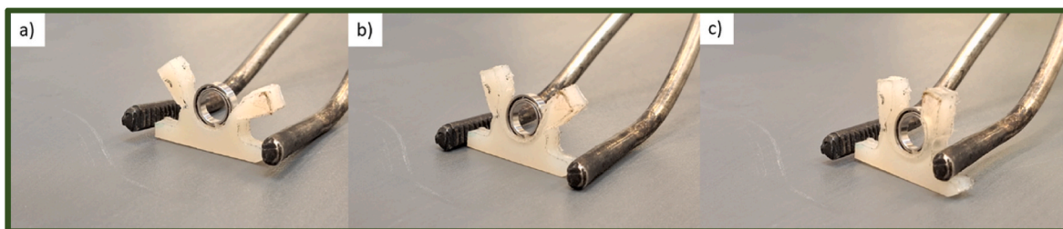
Fig. 9. Demonstration of shape memory on a bearing housing. Programmed shape (a), recovery process (b), and recovered shape (c).
