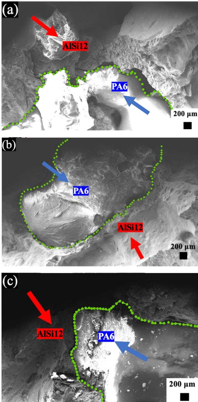
Fig. 3 Metal-PA interface in metal foam-PA composite with different PA content, (a) PA\_1, (b) PA\_3, (c) PA\_5
