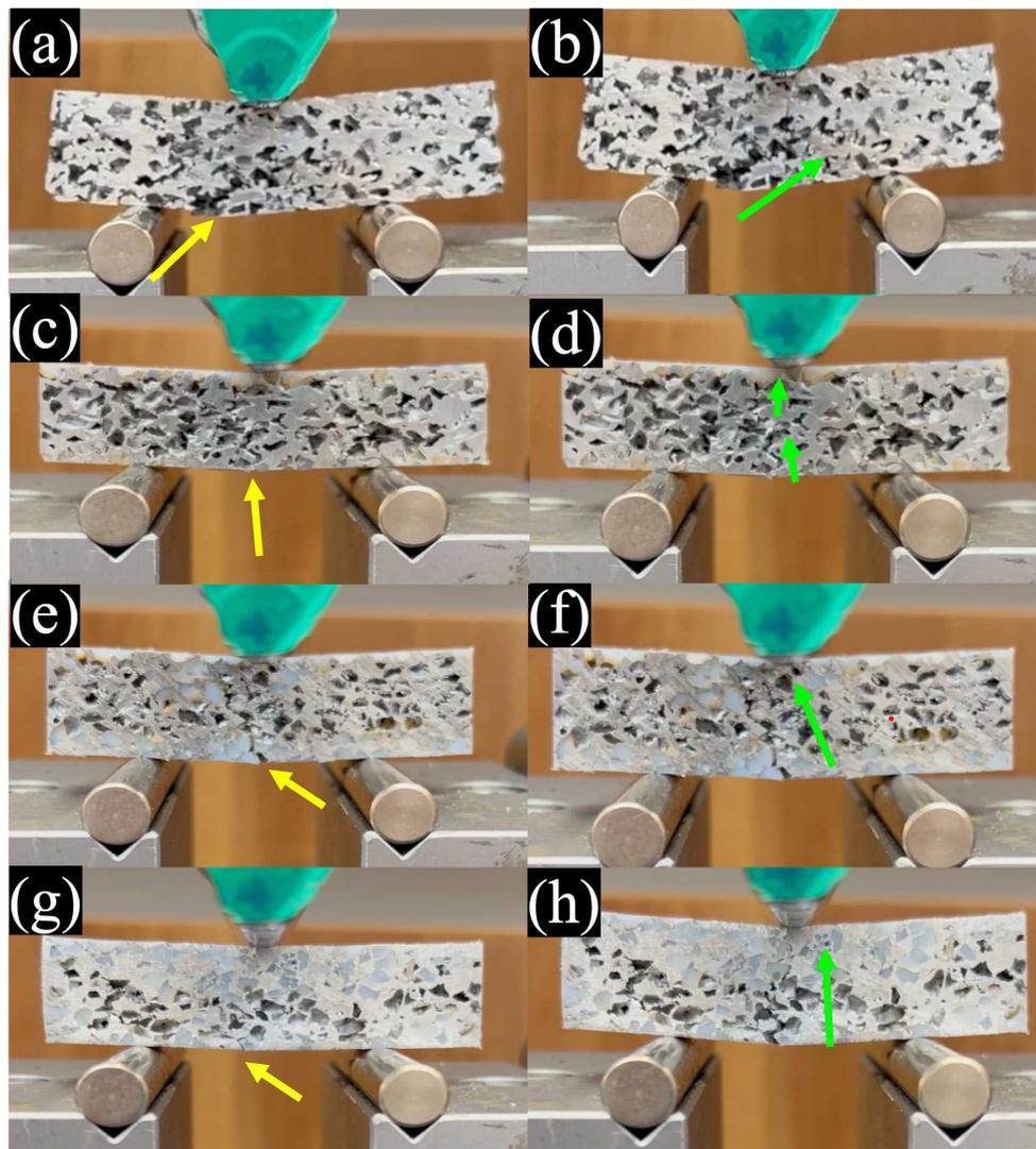
**Fig. 5** The bending behavior of (a) foam at maximum load, (b) foam after removing the load, (c) PA\_1 at maximum load, (d) PA\_1 after removing the load, (e) PA\_3 at maximum load, (f) PA\_3 after removing the load, (g) PA\_5 at maximum load and (h) PA\_5 after removing the load (The yellow and green arrows show the place of crack initiation and the direction of crack propagation, respectively.)
