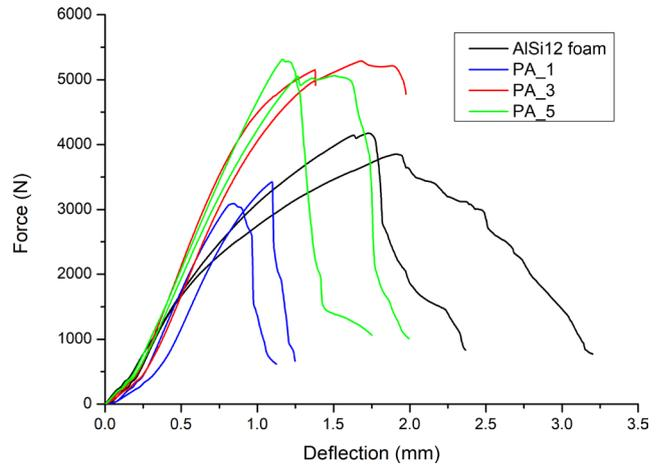
Fig. 4 The load-deflection curves for AISi12 foam (black), PA\_1 (blue), PA\_3 (red) and PA\_5 (green)
