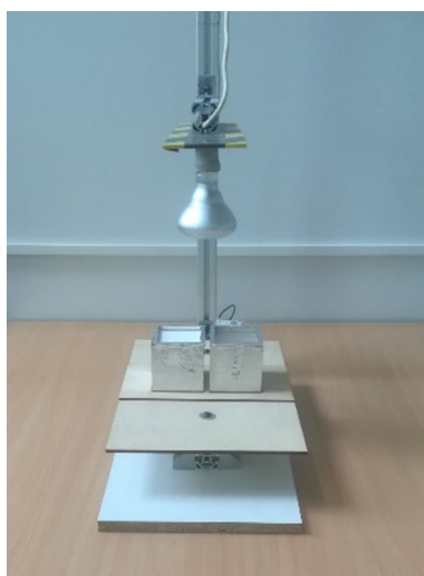
Fig. 1 The arrangement of laboratory-scaled “sun test”
