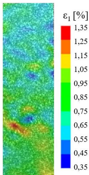
**Figure 16.** Typical strain field of a specimen with 2 mm wide, 0.4 mm thick PCL
