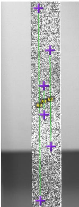
**Figure 9.** Arrangement of the line probe test, A1= 15 mm for local strain measurement, A2=50 mm and A3=75 mm for global strain measurement
