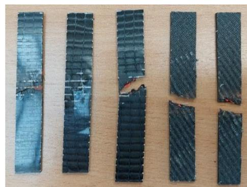
**Figure 5.** The specimens containing PCL interlayer material with a width of 2 mm and a thickness of 0.8 mm after the impact test.
