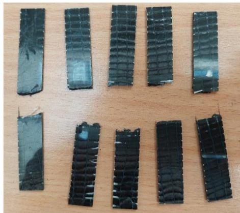
**Figure 3.** Reference specimens after the impact test.
