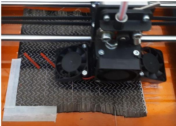
**Figure 1.** Printing of PCL on the UD carbon fabric by FFF method for the impact test specimen.
