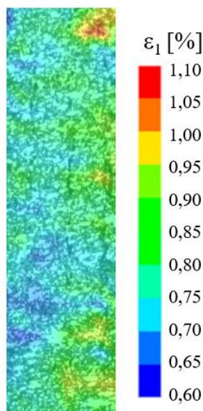
**Figure 14.** Typical strain field of a reference specimen
