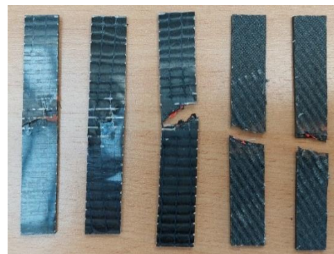
Figure 5. The specimens containing PCL interlayer material with a width of 2 mm and a thickness of 0.8 mm after the impact test.
