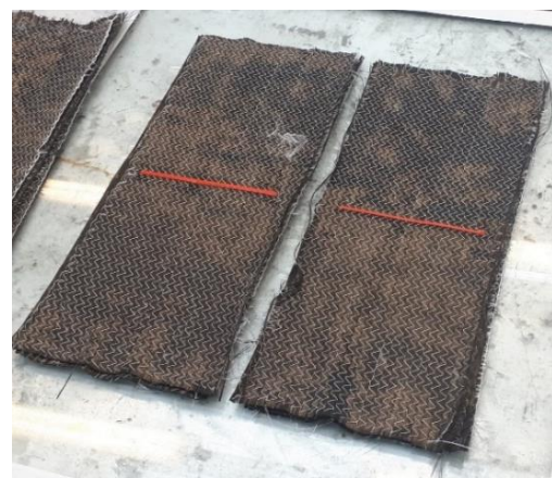
Figure 2. UD carbon fabric containing the PCL interlayer material during the manufacturing of the tensile test specimen.
