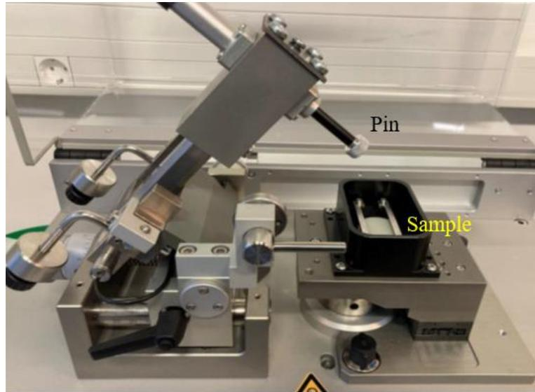
**Figure 5.** Pin-on-disk tribometer
