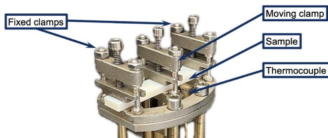
**Fig. 1.** DMA test setup with dual cantilever clamp.
