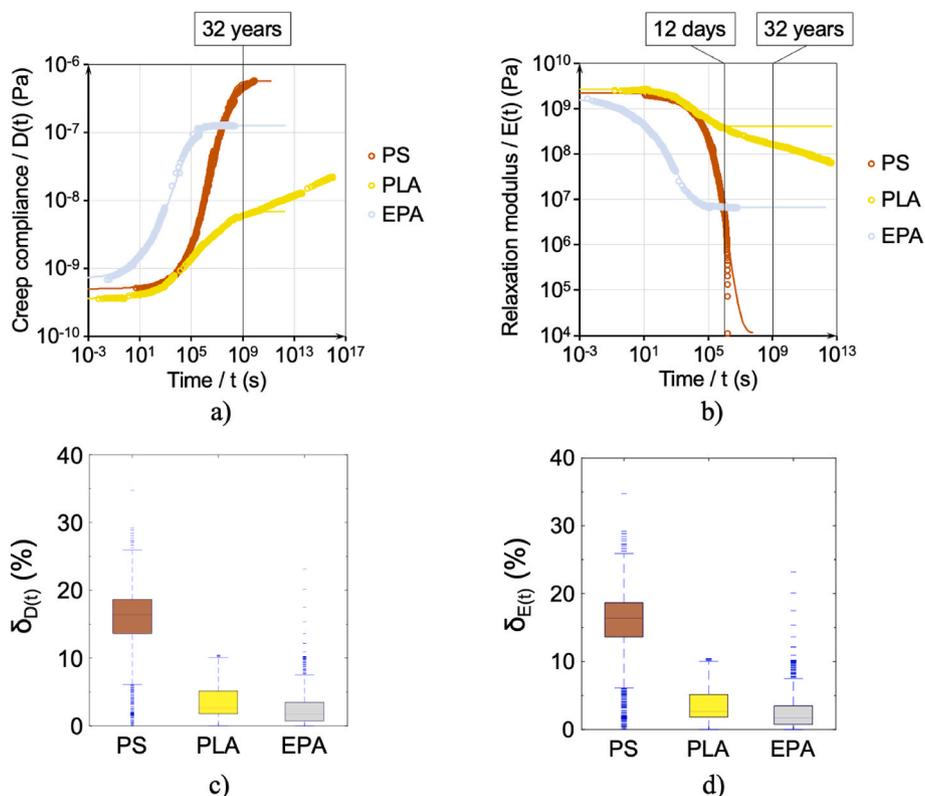
**Fig. 10.** Generated creep compliance (a) and relaxation modulus (b) master curves and models for the amorphous thermoplastic PS, the semi-crystalline thermoplastic PLA, the thermosetting EPA materials in double logarithmic scale, and box plots of percent error for creep (c) and stress relaxation (d) models. The empty circles denote the data points of the TTS curves, and the continuous lines represent the fitted models.
