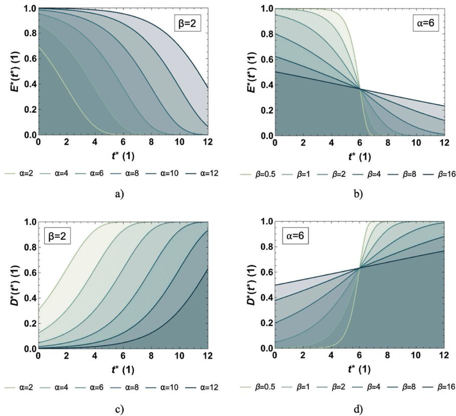
**Fig. 9.** Parametric study of the effect of the location ( $\alpha$ ) and scale ( $\beta$ ) parameters of the Gumbel CCDF (Eq. (7)) (a,b) and the Gumbel CDF (Eq. (8)) models (c,d) using normalised values in double linear scale.
