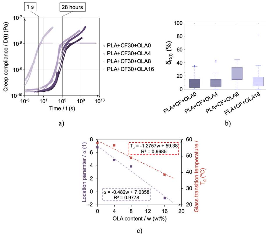
**Fig. 11.** Generated creep compliance master curves and models for plasticised composite materials in double logarithmic scale (a), box plots of percent error for creep models (b) and the quantitative relationship between scale parameter and plasticiser content (c). The empty circles denote the data points of the TTS curves, and the continuous lines represent the fitted models.
