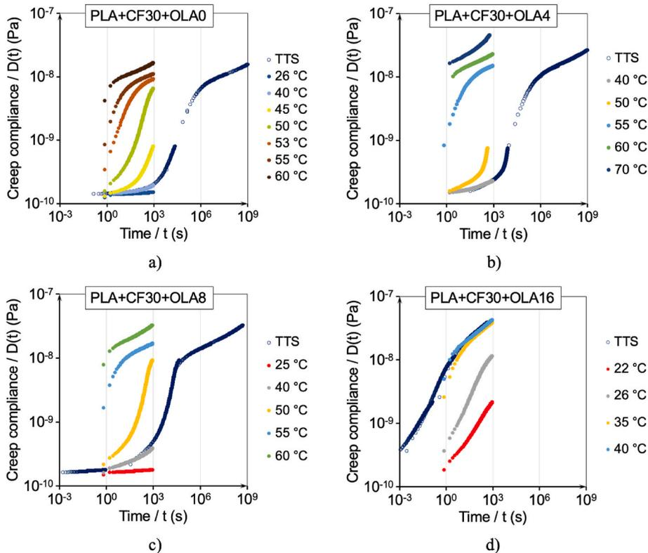
Fig. 6. Master curves generated from creep measurements for the plasticised composites based on the TTS principle at  $T_{ref} = 40\text{ }^{\circ}\text{C}$  in double logarithmic scale.
