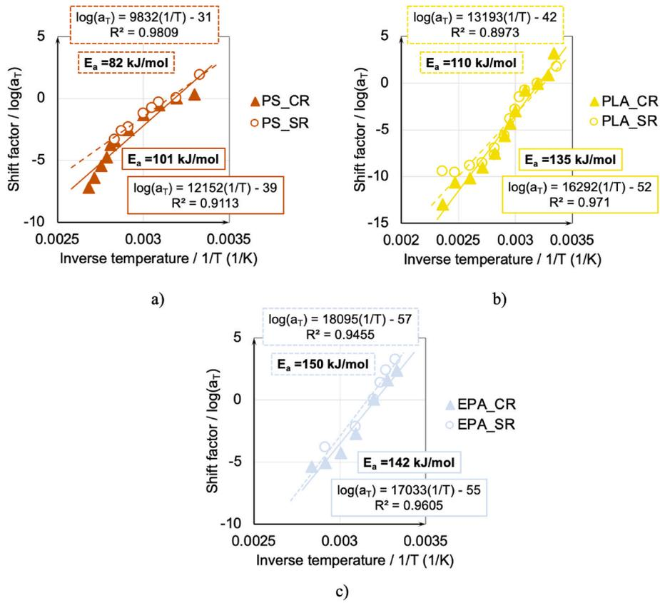
**Fig. 4.** Arrhenius plots of the shift factors used to generate the creep compliance and relaxation modulus master curves for the amorphous thermoplastic PS (a), the semi-crystalline thermoplastic PLA (b) and the thermosetting EPA (c) in double linear scale. Full markers and continuous lines stand for creep (CR), and empty markers and dashed lines stand for stress relaxation (SR).
