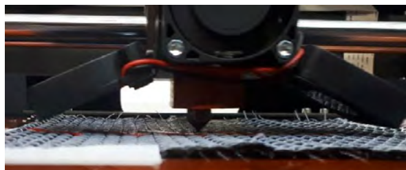
Figure 1. 3D printing of PCL interlayer material on the reinforcement fabric using FFF method
