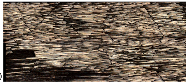
Fig. 4.17. Compressive behaviour of [\pm 27/0]_S MR60/M55J carbon layup, a) Pseudo-ductile stress-strain response and b) compressive ply fragmentation in the central 0^\circ plies [178].
