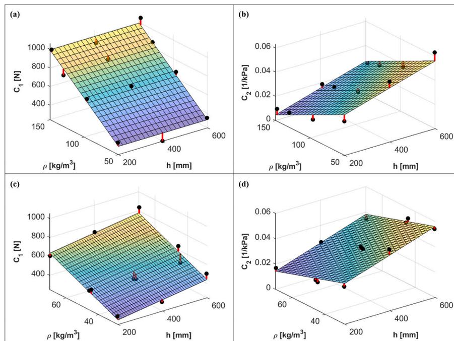
**Fig. 7.** Multiple linear regression of the  $C_1$  (a) and  $C_2$  (b) coefficients for EVA; the multiple linear regression of the  $C_1$  (c) and  $C_2$  (d) coefficients for XPE, residuals illustrated with red lines. (For interpretation of the references to colour in this figure legend, the reader is referred to the Web version of this article.)
