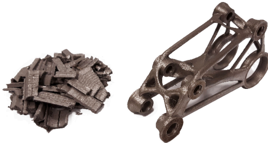
Fig. 15. The printed model and the removed support after detaching from the building platform.
