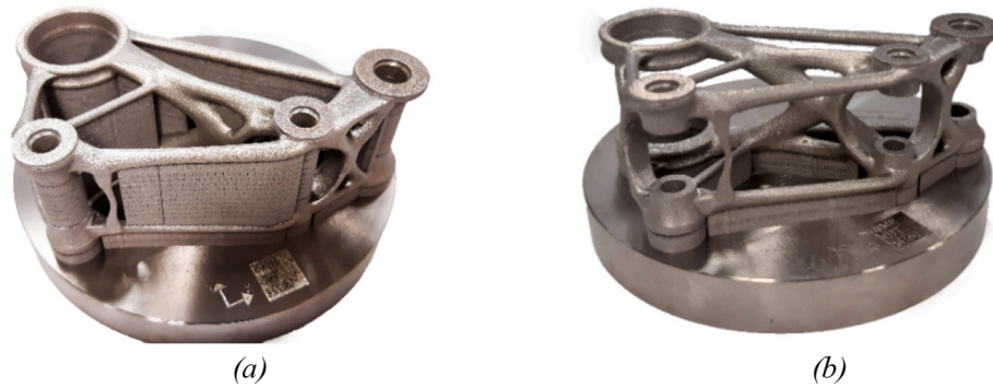
Fig. 14. The printed model fixed on the building platform (a) with inner supports, (b) without inner supports.
