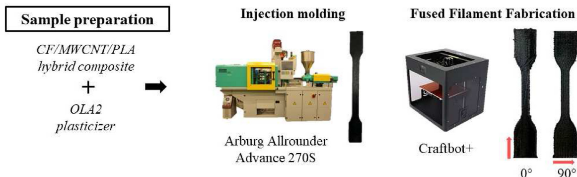
Figure 2. Production of tensile samples by injection molding and fused filament fabrication.
