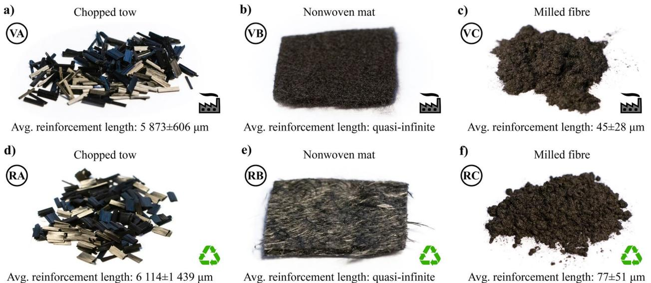
**Fig. 1** The six different fibre reinforcement types used in this study: **a** virgin chopped fibres, **b** virgin nonwoven mat, **c** virgin milled fibres, **d** recycled chopped fibres, **e** recycled nonwoven mat, and **f** recycled milled carbon fibres
