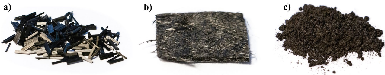
Fig. 1 The different structures of fibre reinforcements used: (a) chopped carbon fibres, (b) nonwoven mat and (c) milled carbon fibres
