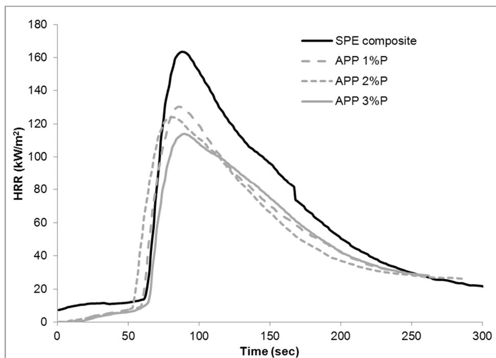
**Figure 3.** Heat release rate of reference and flame retarded SPE composites with ammonium polyphosphate (APP).
