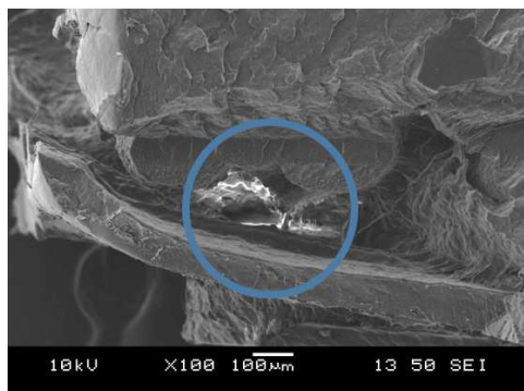
Fig. 4. FFF printed UHMWPE first layer at 100x magnification
