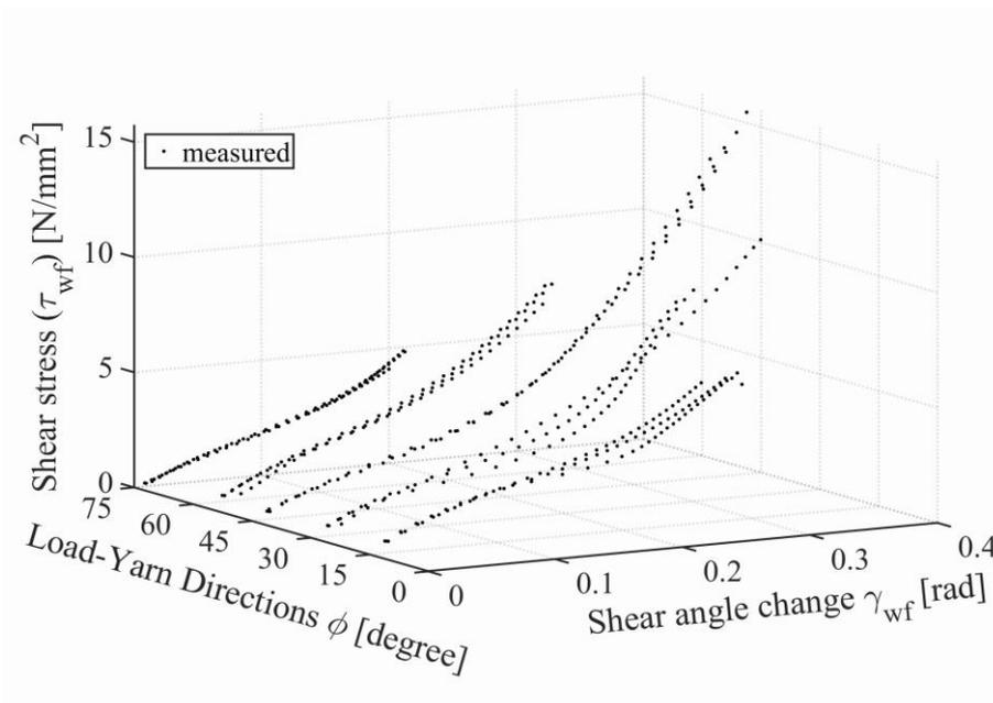
**Figure 11.** The measured stress-strain curves for shear with respect to the angle of the load ( $\phi$ ) in the  $\gamma_{wf} - \tau_{xy} - \phi$  coordinate system.
