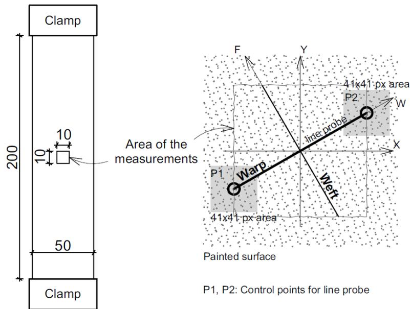
**Figure 8.** The defined line probe and correlation interval area around its control points.
