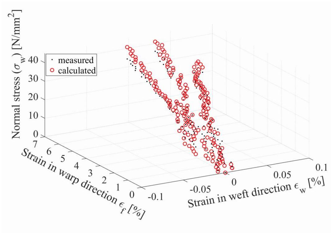
**Figure 3.** The representation of the result of the parameter identification for the warp stress direction by the function of the bi-axial strains.
