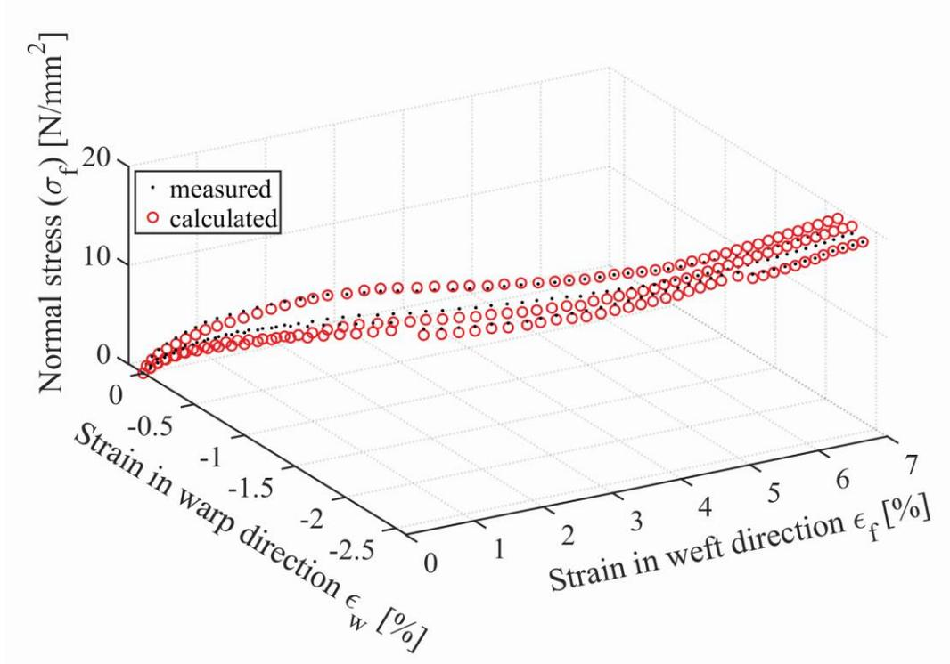
**Figure 4.** The representation of the result of the parameter identification for the weft stress direction by the function of the bi-axial strains.
