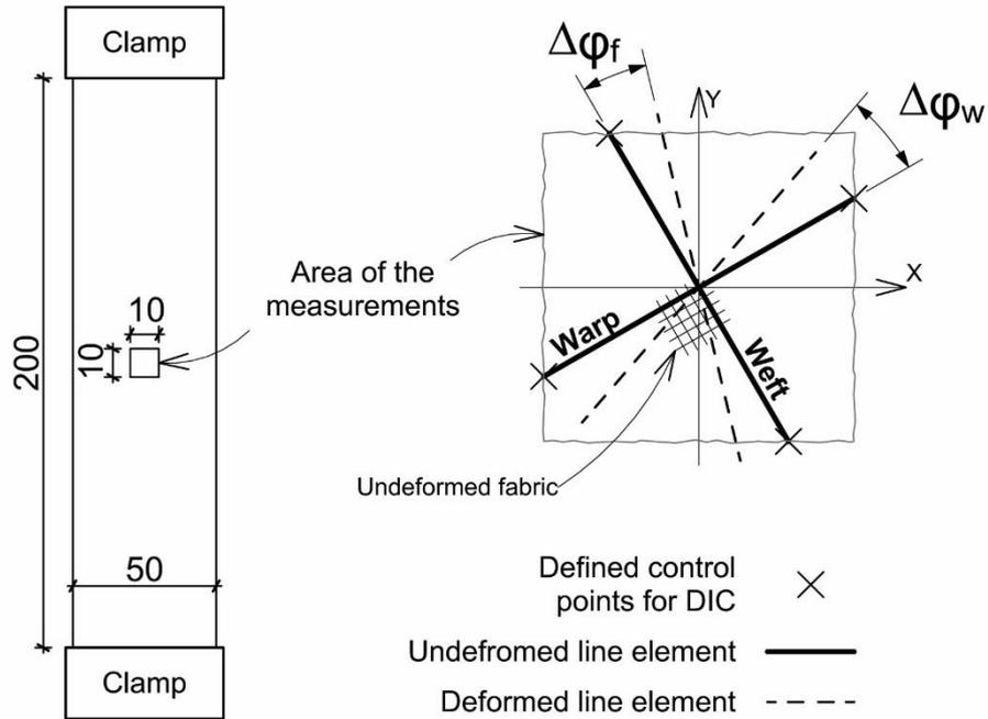
**Figure 9.** The measured strains for the determination of the shear modulus during the test.
