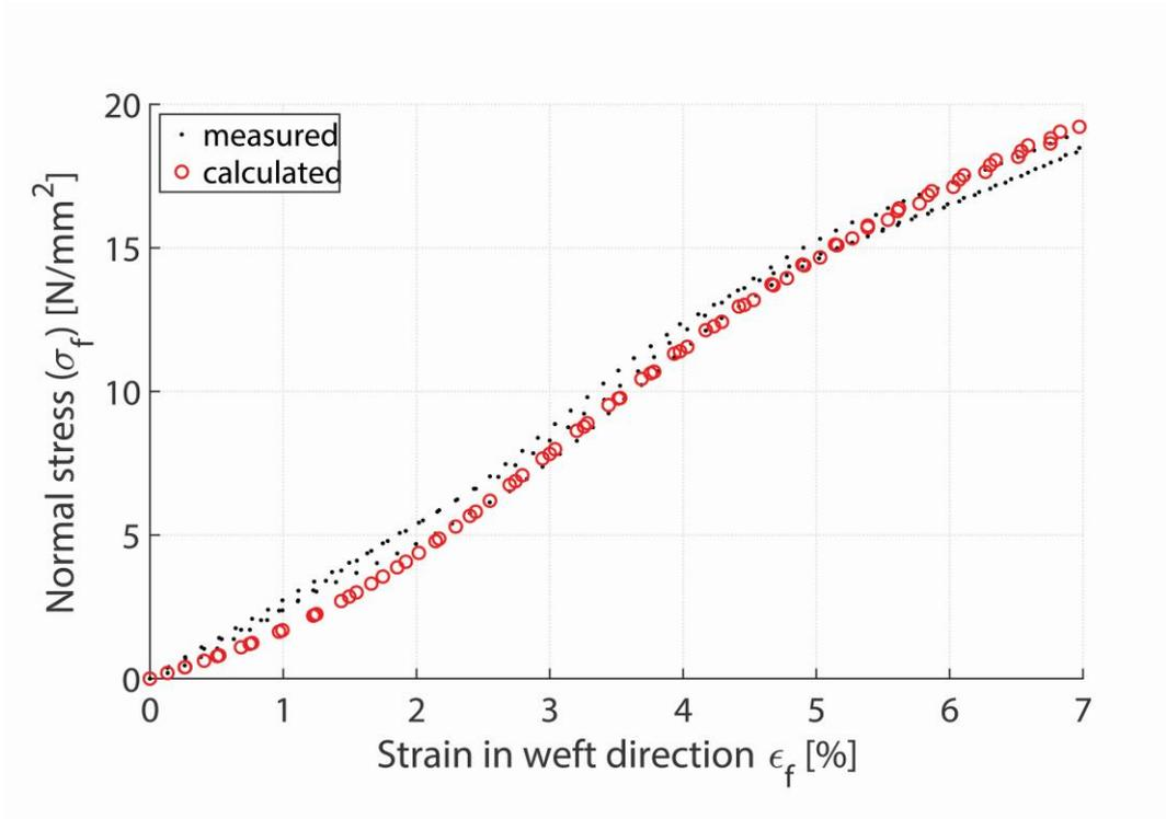
**Figure 2.** The uniaxial projection of the result of the parameter identification for the weft direction for PVC coated textile.
