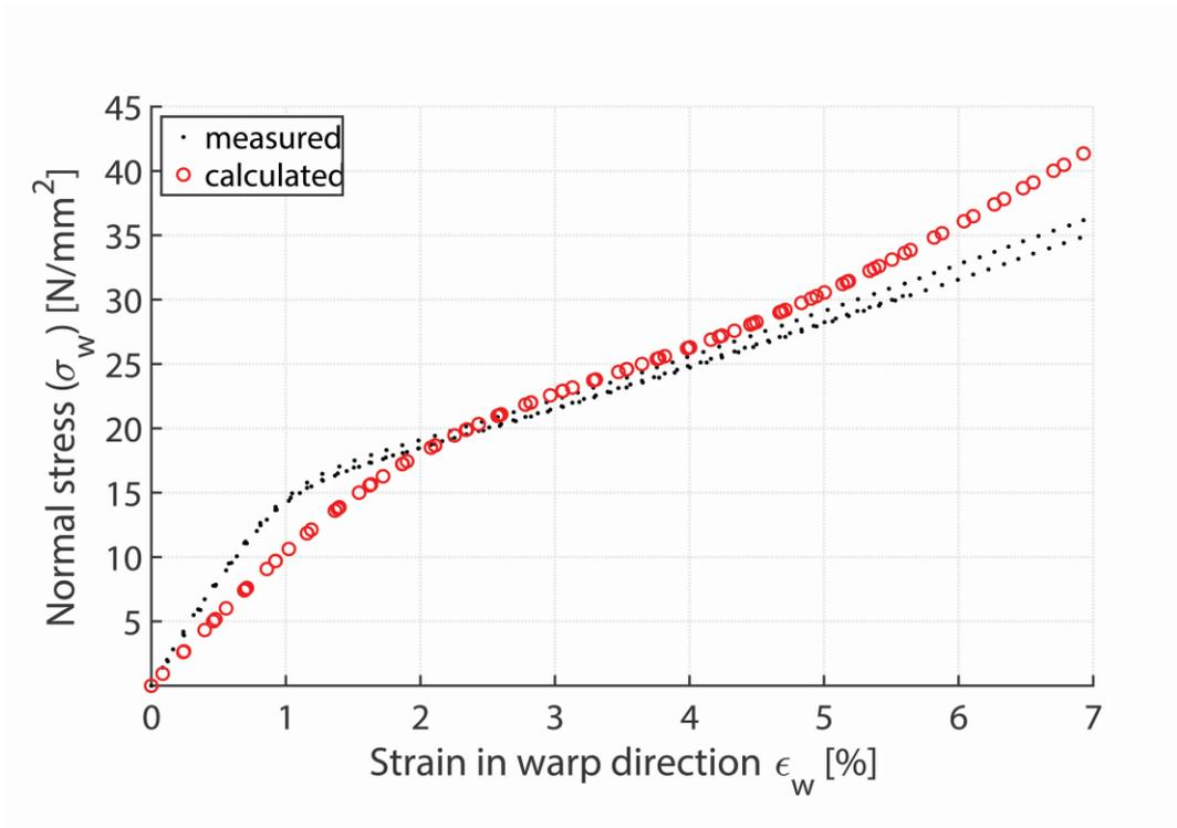
**Figure 1.** The uniaxial projection of the result of the parameter identification for the warp direction for PVC coated textile.
