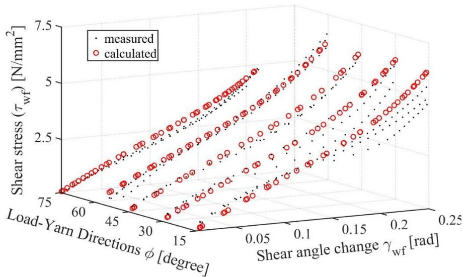
**Figure 12.** The measured and fitted  $\tau_{wf}$  shear stress values in function of  $\gamma_{wf}$  and  $\phi$ , ( $R^2 = 0.977$ )
