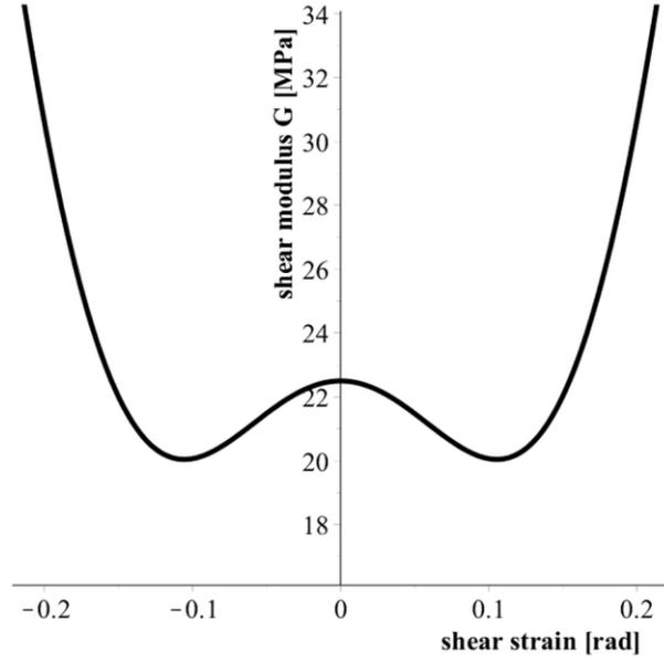
**Figure 13.** The value of the shear modulus in the examined range of shear strains.
