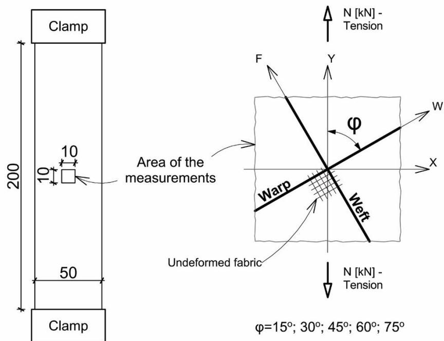
**Figure 5.** The experimental arrangement of the test strips
