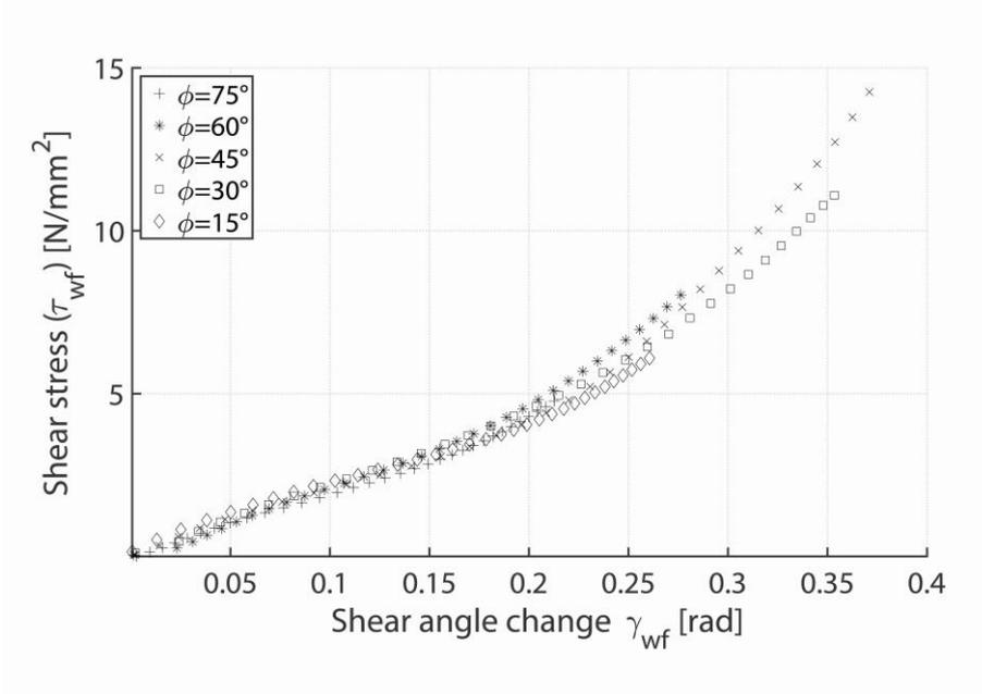
**Figure 10.** The projection of one measured shear stress-strain curves from each load directions projected to the  $\gamma_{wf} - \tau_{xy}$  coordinate system.
