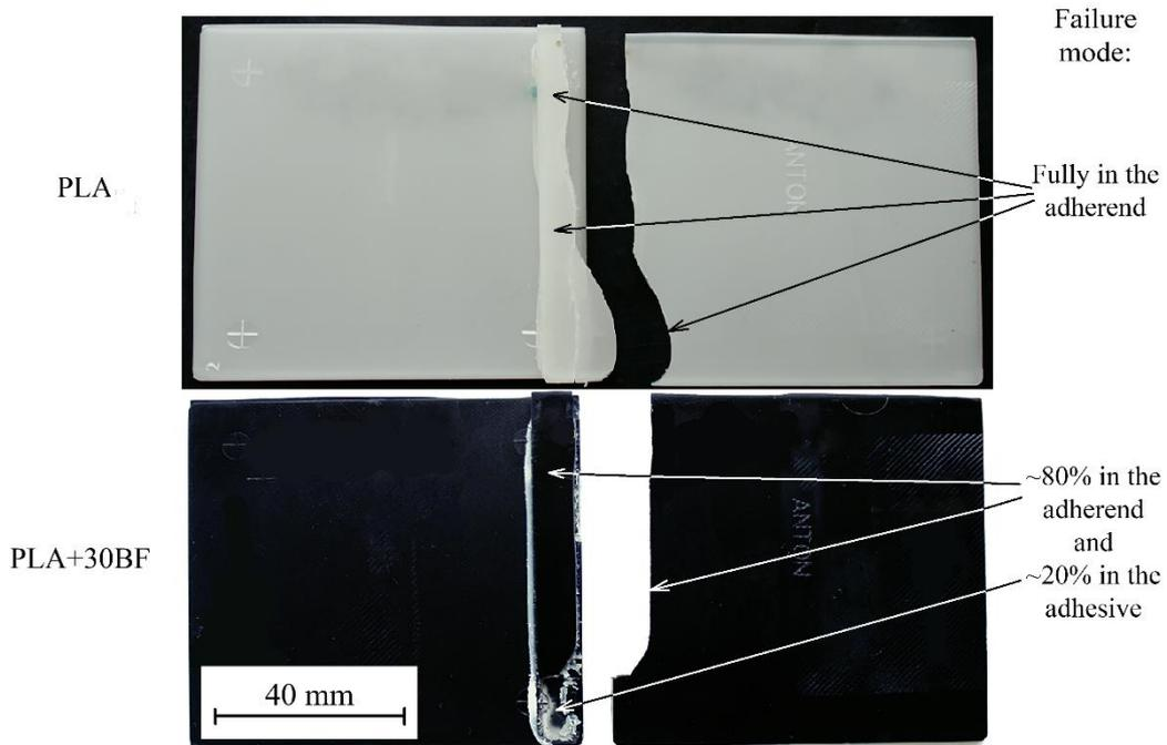
Figure 3. Tensile tested thin sheets of pure PLA and PLA+30BF joined together with acrylate-based adhesives
