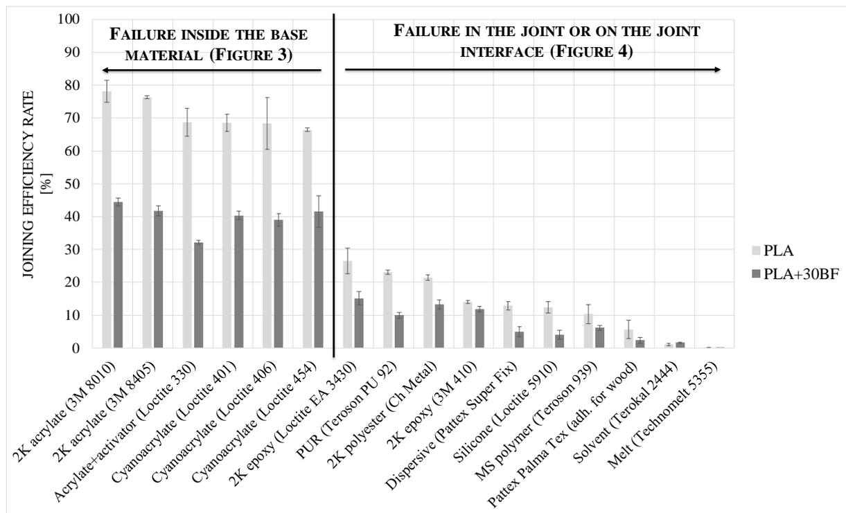
Figure 2. Joining efficiency rates of adhesive bonded specimens
