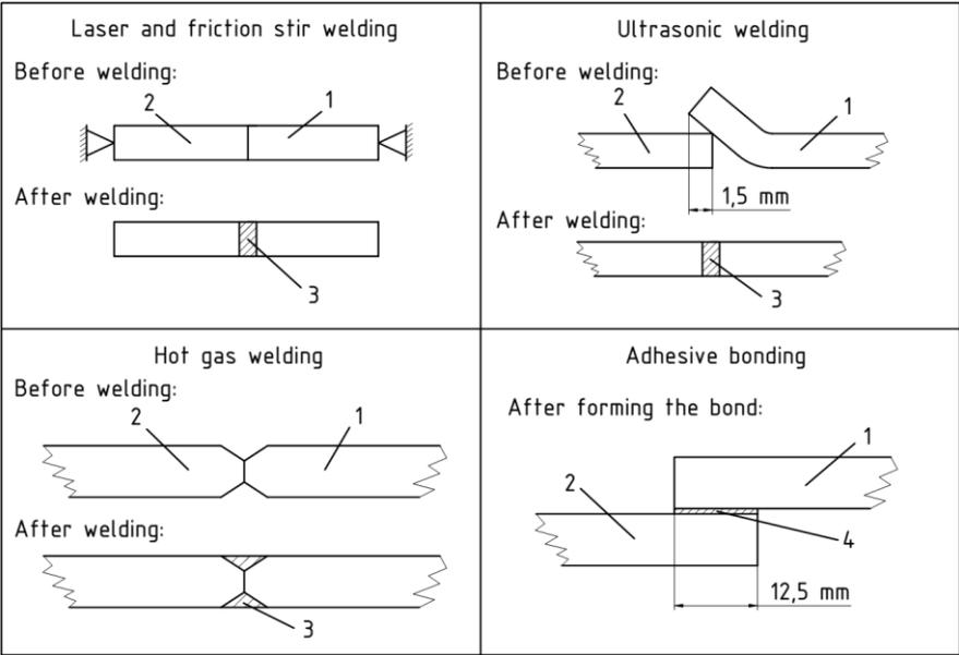
Figure 1. The illustration of bonds (Legend: 1-2 Adherends, 3 Bond, 4 Joint)
