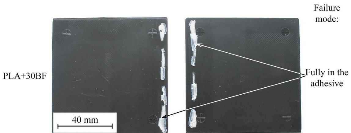
Figure 4. Tensile tested thin sheets of PLA+30BF joined together with a dispersion adhesive
