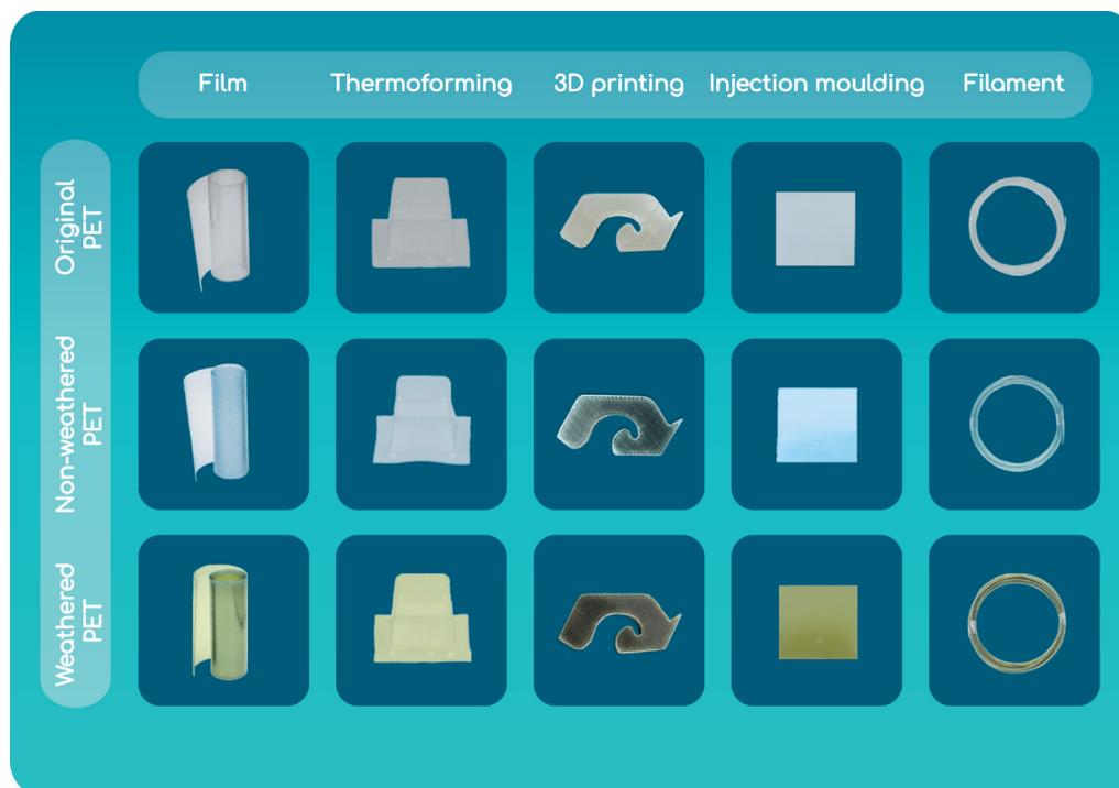
Fig. 5. Products manufactured by different technologies, made from original, non-weathered PET and weathered PET.
