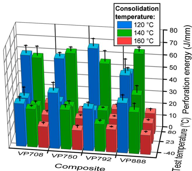
Fig. 11. Perforation energy of the composites.
