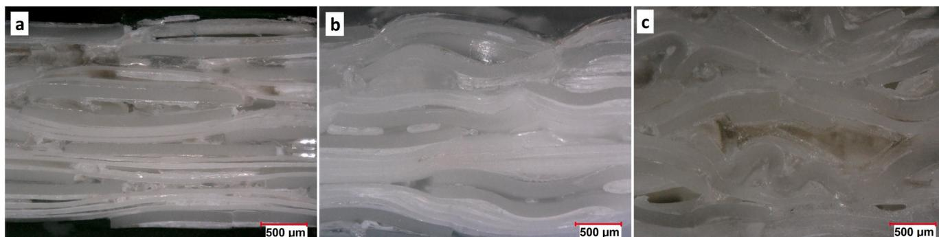
Fig. 5. Light microscopic images of VP792 composite consolidated at 120 °C (a), 140 °C (b), and 160 °C (c).
