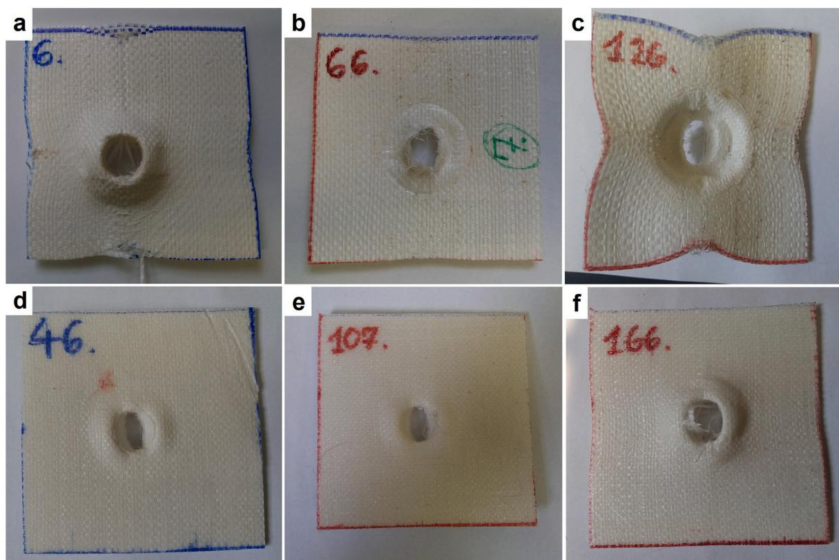
Fig. 10. Typical failure behavior of composites with Fabric 1 and the VP750 matrix consolidated at 120 °C at the test temperatures of -40 °C (a), 23 °C (b), and 80 °C (c) and the composites with the same components consolidated at 160 °C at the test temperatures of -40 °C (d), 23 °C (e) and 80 °C (f).
