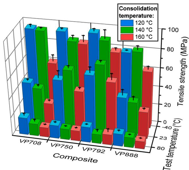
Fig. 7. Tensile strength of the composites.
