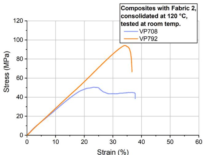
Fig. 8. Typical tensile curves of the composites made with Fabric 2.
