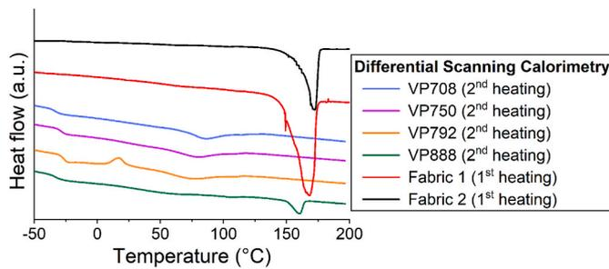
Fig. 3. DSC curves of the reinforcements and matrices, obtained from the 1st heating cycle for the fabrics, and 2nd heating cycle for the matrices.
