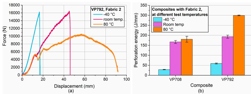
Fig. 13. Typical IFWI curves of the VP792 composite made with Fabric 2 (a) and perforation energy of the composites produced with Fabric 2 (b) at different test temperatures.
