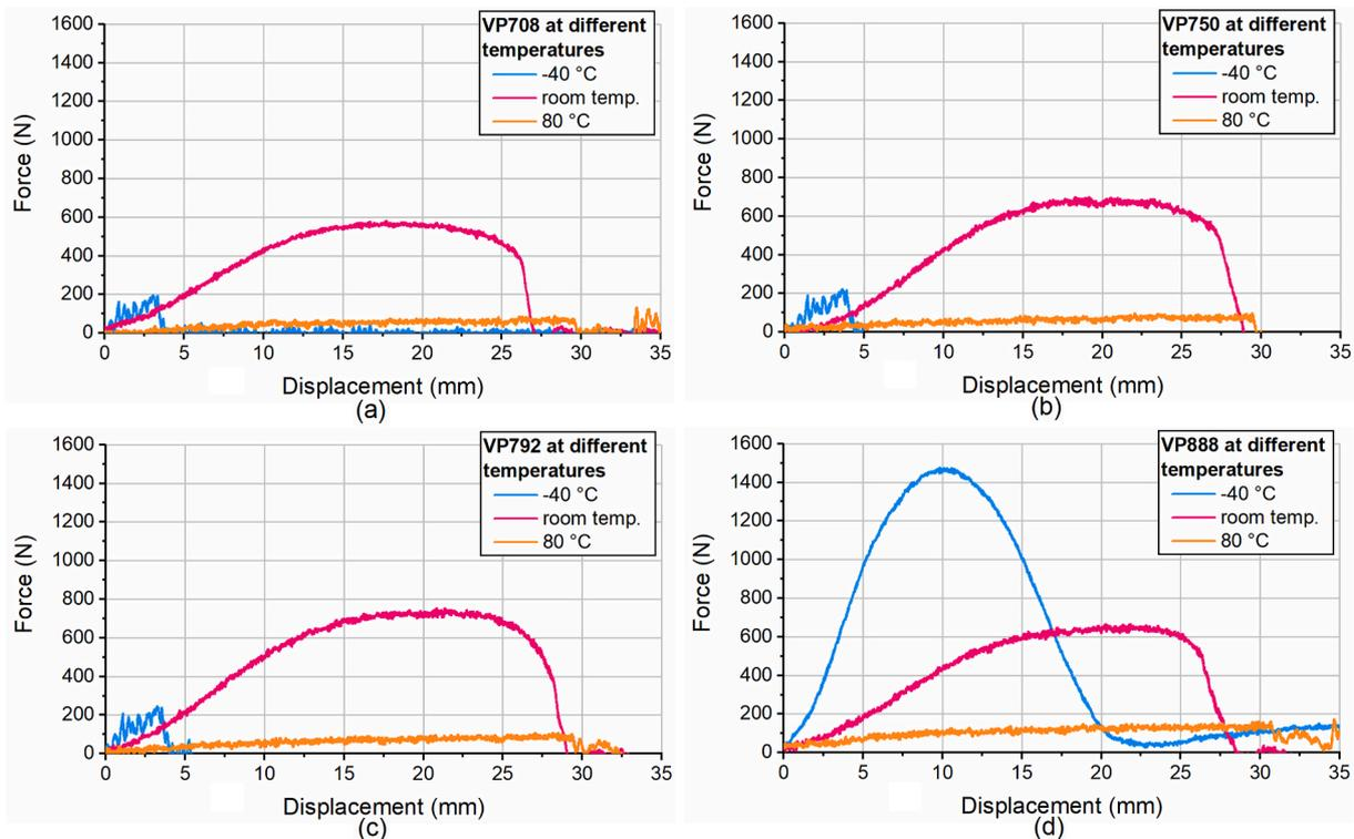
Fig. 4. Typical IFWI curves of VP 708 (a), VP750 (b), VP792 (c), and VP888 (d) matrices at different test temperatures.
