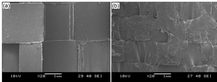
Fig. 12. Scanning electron microscopic pictures of the VP792 composite consolidated at 120 °C (a) and 160 °C (b).
