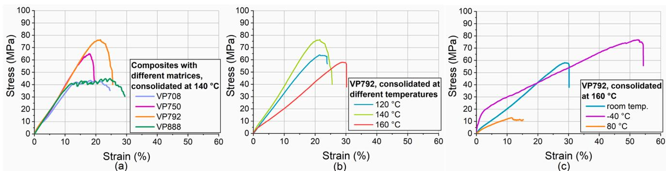
Fig. 6. Typical tensile curves of the composites with different matrices consolidated at 140 °C tested at room temperature (a), the effects of consolidation temperature (b) and the effects of test temperature (c).
