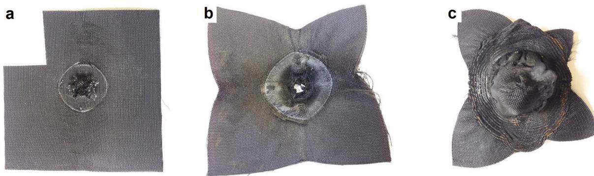
Fig. 14. Typical failure behavior of composites with Fabric 2 and the VP 708 matrix at the test temperatures of  $-40$  °C (a),  $23$  °C (b), and  $80$  °C (c).
