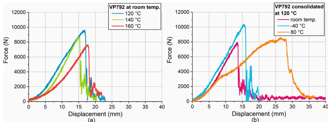
Fig. 9. Typical IFWI curves of the VP792 composites tested at room temperature (a), and the effect of the test temperature (b).
