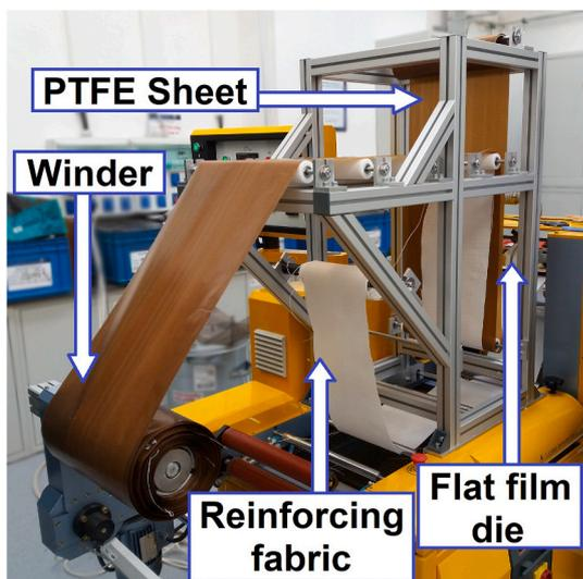
Fig. 2. The custom-built fabric-conveying apparatus.
