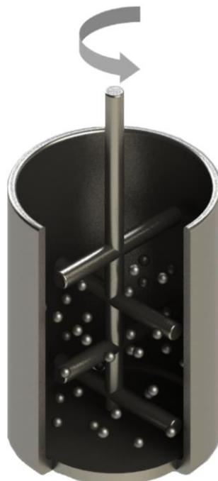
**Figure 1.** Schematic build-up of the attritor
