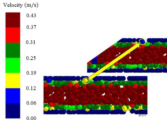
**Figure 8.** The anomaly of the filler particles in the model
