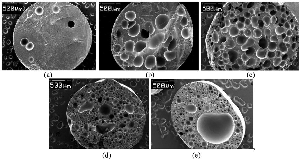
**Figure 1.** SEM images of PLA foams produced with a) 0.5 wt%, b) 1 wt%, c) 2 wt%, d) 4 wt%, e) 8 wt% exothermic chemical blowing agent at the same manufacturing temperature (190 °C); magnification is 30x
