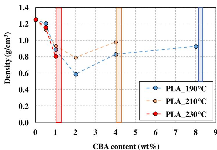
**Figure 5.** The density of foams as a function of CBA content at different production temperatures (190 °C, 210 °C and 230 °C); blue line: production limit at 190 °C; orange line: production limit at 210 °C; red line: production limit at 230 °C
