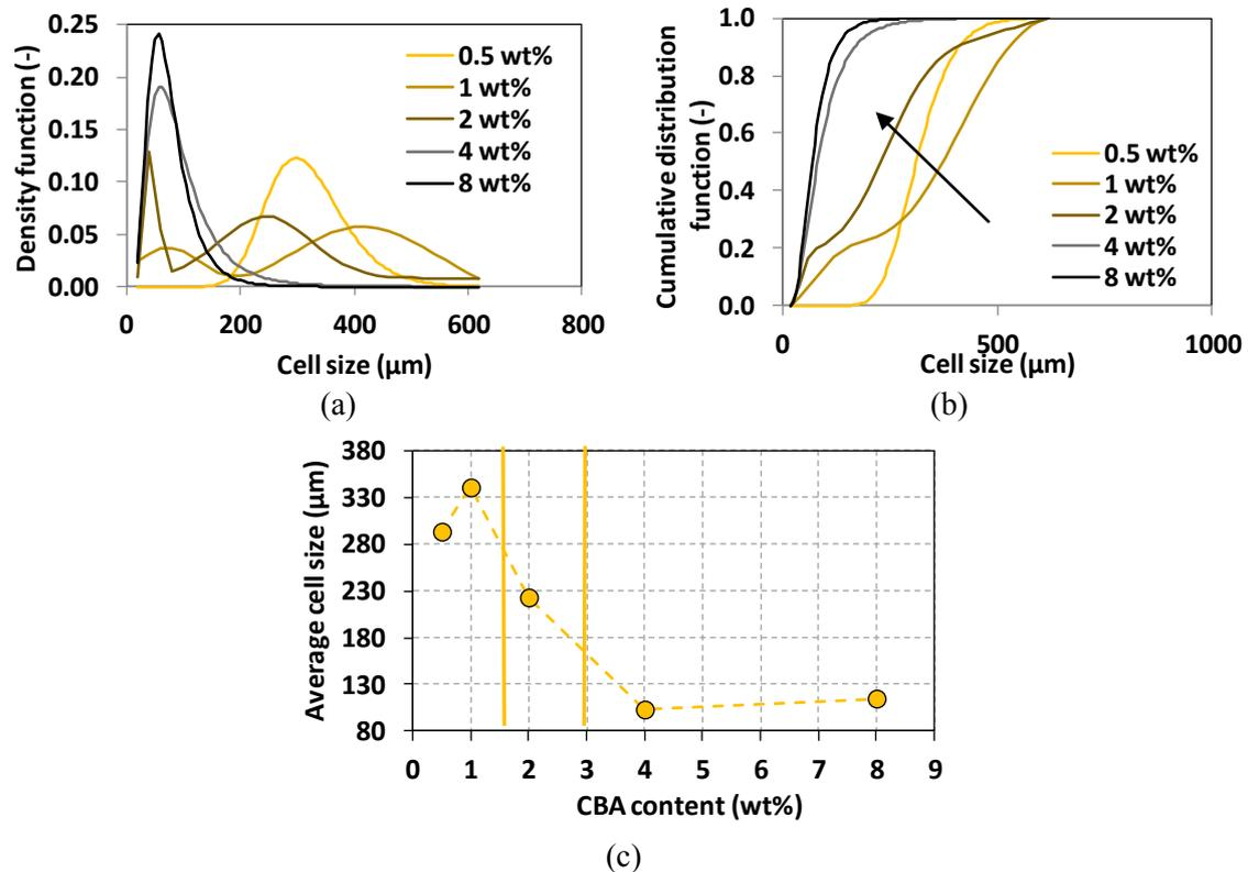
**Figure 2.** Calculated values of foam structures containing exothermic CBA a) density function as a function of cell size (8 wt% CBA), b) Cumulative distribution function and c) average cell size as a function of CBA content
