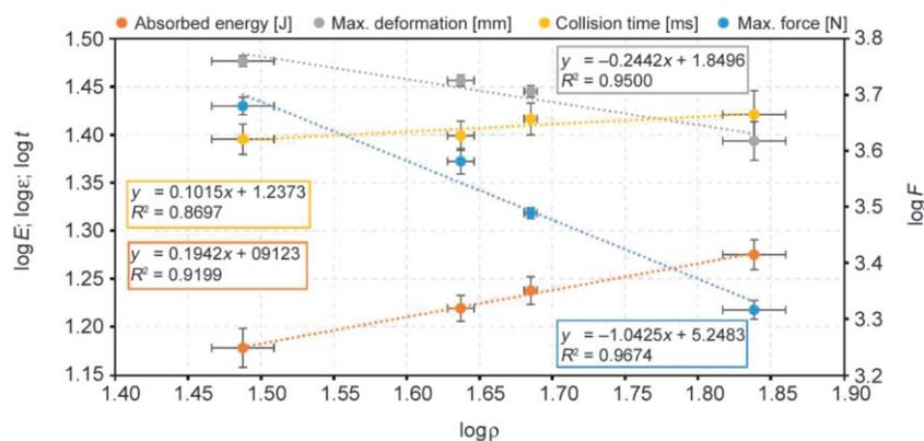
**Figure 4.** The relationship between absorbed energy, maximum force, maximum deformation, collision time, and density [kg/m<sup>3</sup>].
