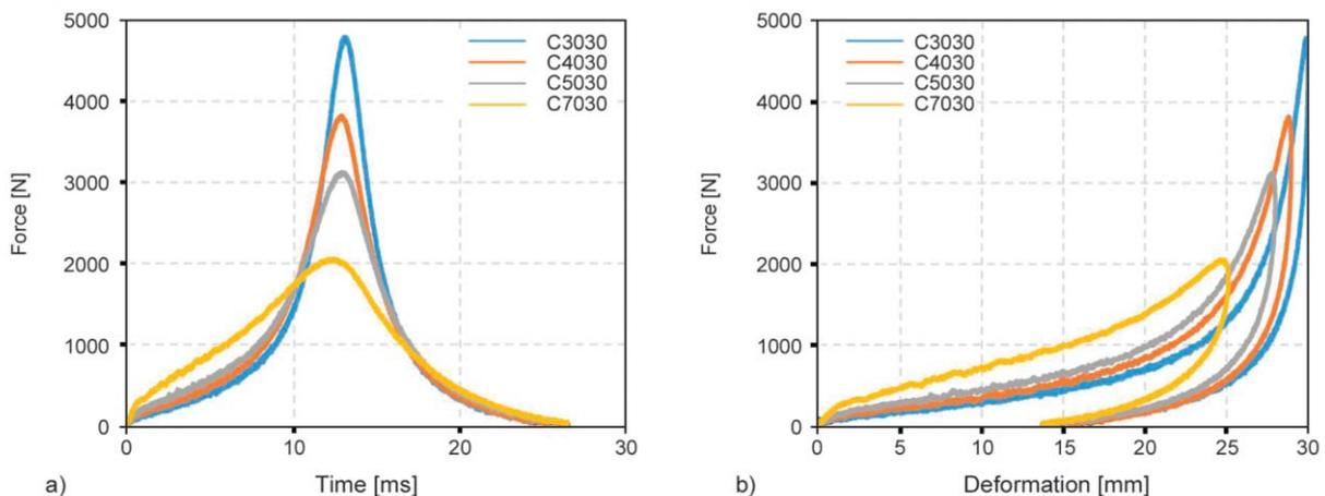
Figure 3. Force-time (a) and force-deformation (b) curves of the falling weight tests.
