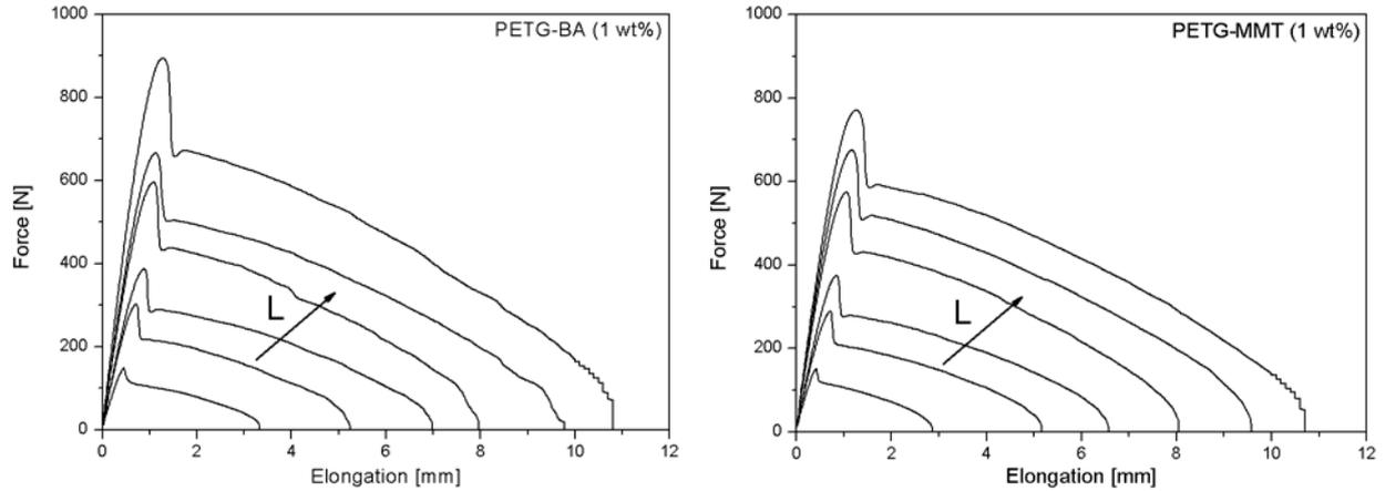
Figure 4. F-x traces as a function of the ligament length (L) measured on DEN-T specimens of PETG-BA (a) and PETG-MMT nanocomposites (b).
