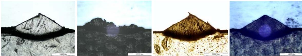
Figure 6. LM pictures taken from the failed DEN-T specimens of the neat PETG, and its nanocomposites containing GR, BA and MMT, respectively (from left to right)
