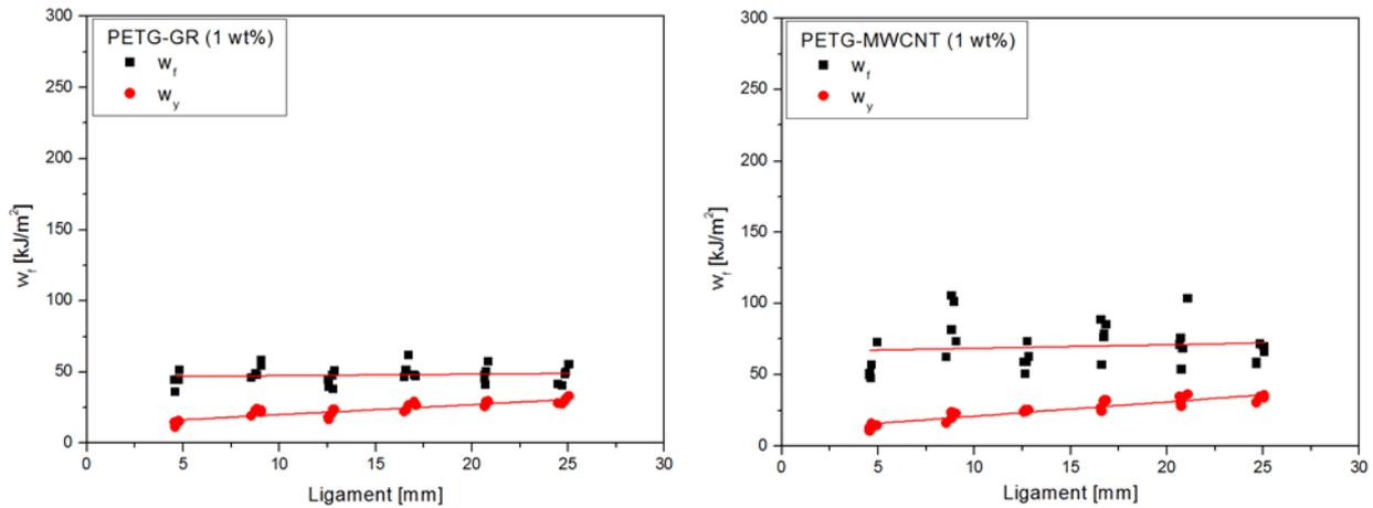
Figure 3.  $w_f$ - $L$  traces as a function of the ligament length ( $L$ ) measured on DEN-T specimens of PETG-GR (a) and PETG-MWCNT (b).
