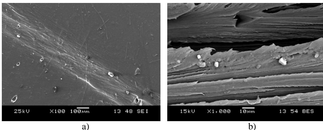
Figure 7. SEM pictures from the surface of the transition between the plastic zone (bottom left) and bulk (top right) (a) and from the fracture zone (b) of a DEN-T specimen of PETG-BA
