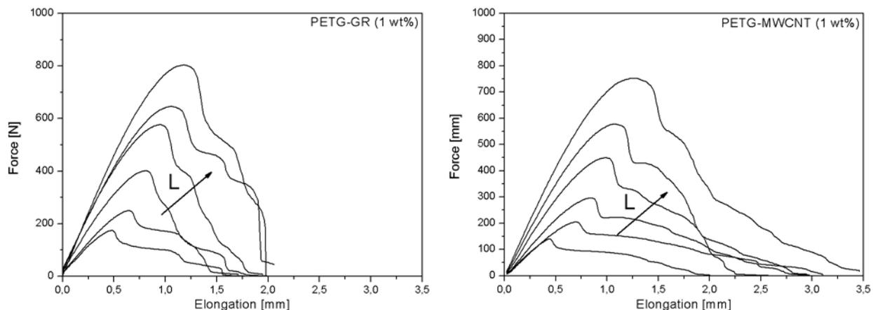
Figure 2.  $F$ - $x$  traces as a function of the ligament length ( $L$ ) measured on DEN-T specimens of PETG-GR (a) and PETG-MWCNT (b).
