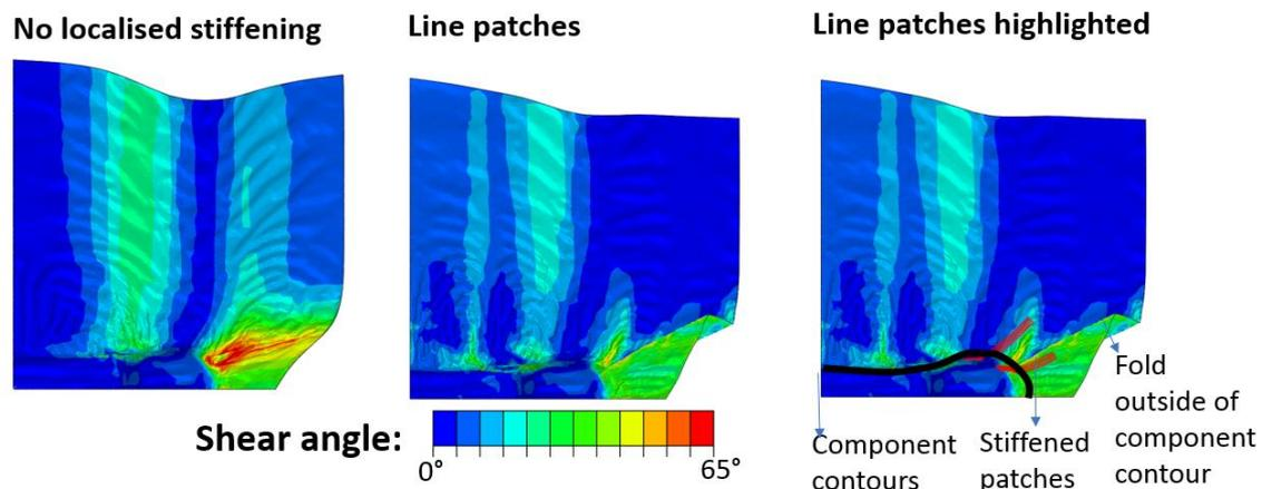
**Figure 7.** Forming simulations with and without stabilising patches
