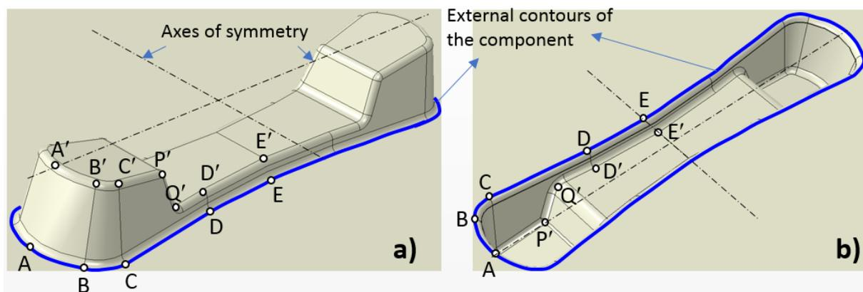
**Figure 1.** Geometry of the a) male and b) female moulds of the component.
