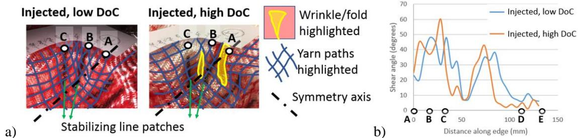
**Figure 6.** a) Deformation of the formed fabric with different line treatments, b) Shear angle along the edge A-B-C-D-E (see Fig. 1 for references).
