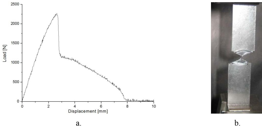
Figure 5. Load-displacement curves and macroscopic failure behavior for the matrix material
