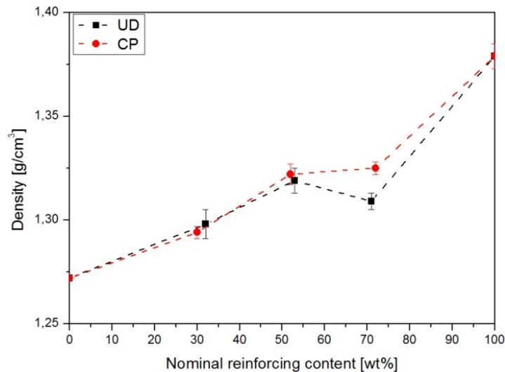
**Figure 1.** Density of the cross-ply and unidirectional composites as a function of reinforcing content. Note that the density at 100 wt% was determined on the reinforcing fibers
