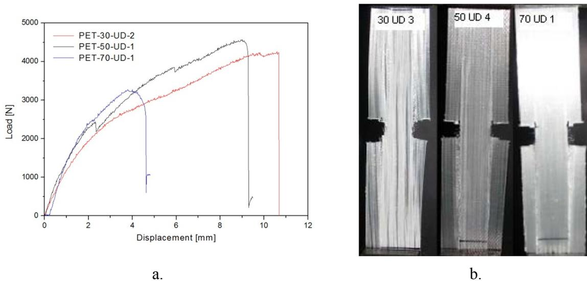
Figure 6. Load-displacement curves (a) and macroscopic failure behavior (b) for cross-ply PET composites
