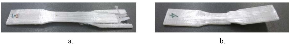
**Figure 4.** Typical macroscopic failure behavior of tensile specimens – 50 wt% UD (a) and 50 wt% CP (b)
