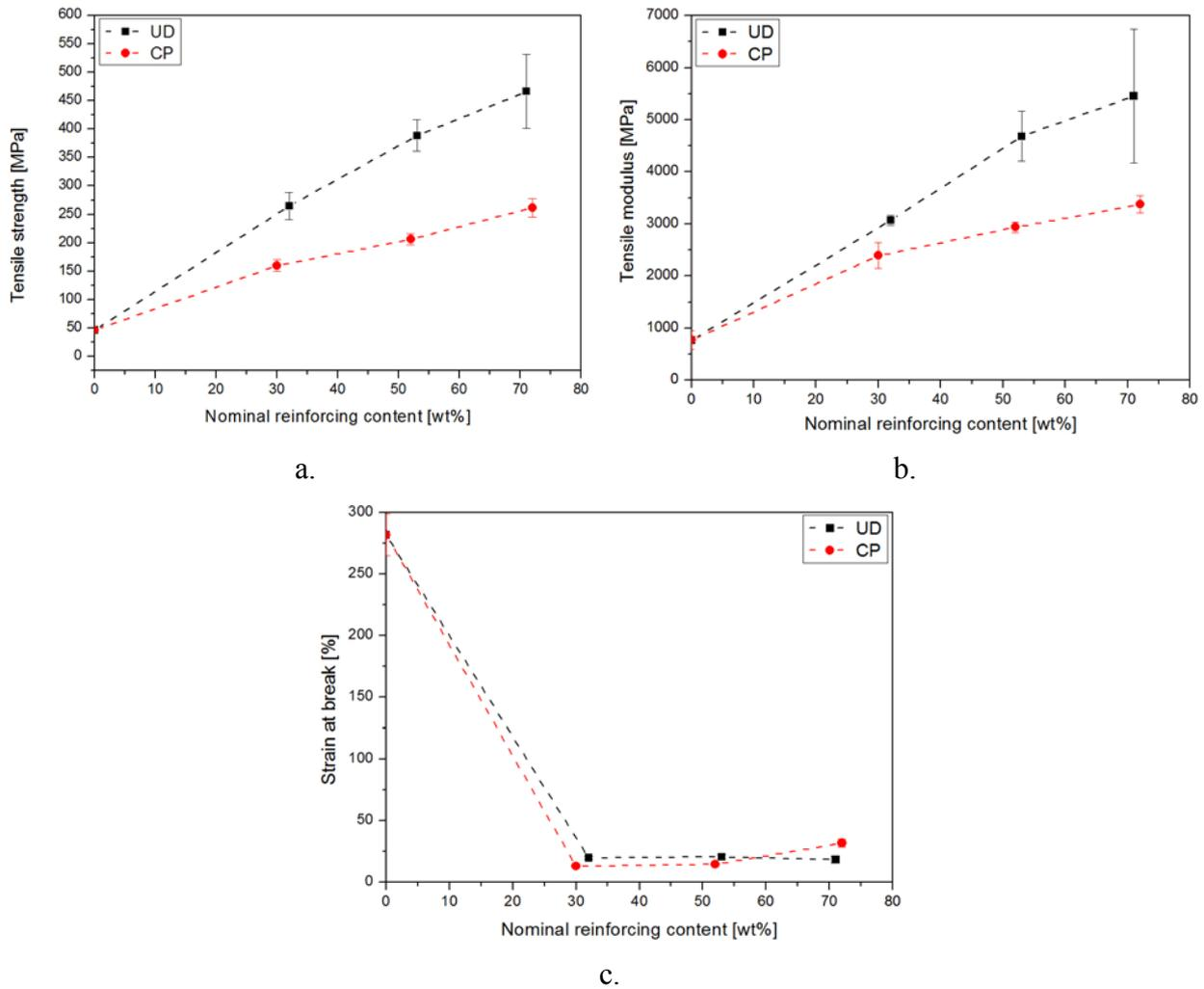
**Figure 3.** Tensile strength (a), tensile modulus (b) and elongation at break values for the cross-ply and unidirectional composites as a function of nominal reinforcing content.
