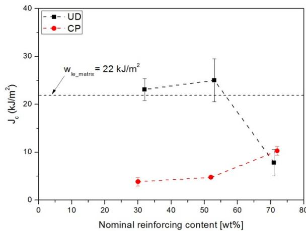
**Figure 8.** Toughness-reinforcing content curves for CP and UD all-PET composites
