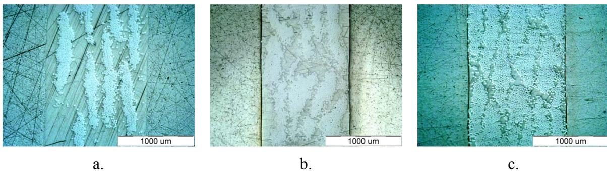
**Figure 2.** LM pictures taken from the polished cross section of UD composites having a reinforcing content of 30 (a), 50 (b) and 70 wt%
