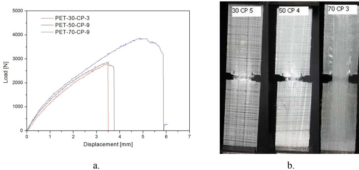
**Figure 7.** Load-displacement curves (a) and macroscopic failure behavior (b) for unidirectional PET composites
