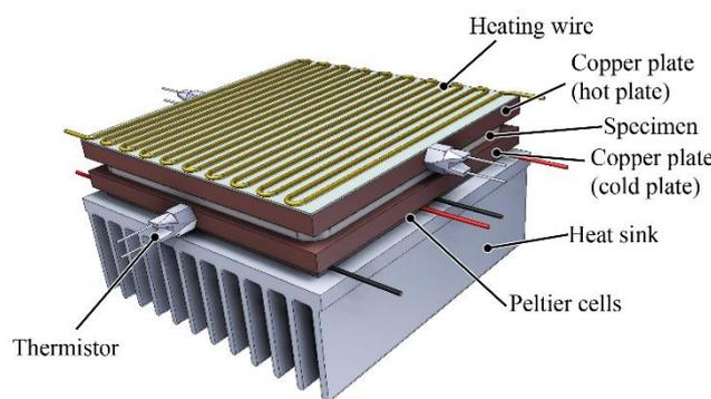
**Figure 2.** Assembly of the hot-plate measuring unit without thermal insulation.
