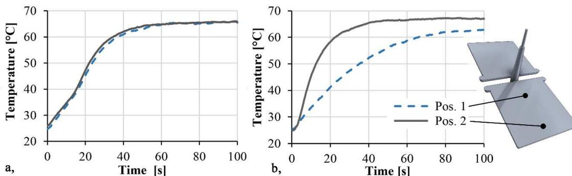
**Figure 10.** Heating curves of the injection-molded 20 vol % GB filled samples (a, GB size: 45–75 μm; b, 120–165 μm).
