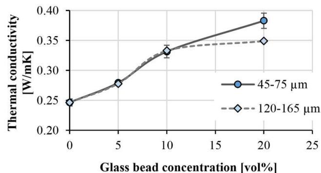
**Figure 9.** Thermal conductivity of filled polypropylenes.
