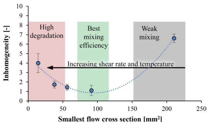
**Fig. 8.** The homogeneity of the samples as a function of the smallest flow cross section.
