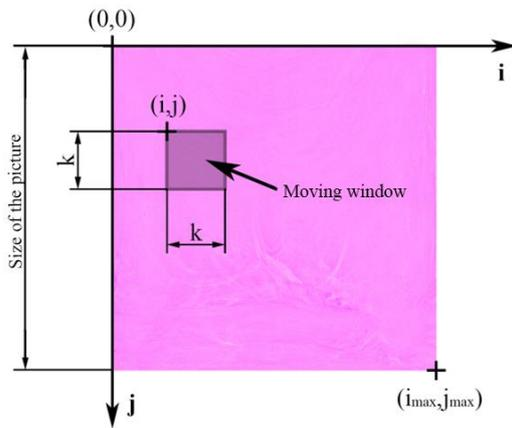
**Fig. 1.** Digitized image of a test specimen and the measuring method with the moving window
