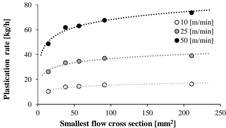
**Fig. 4.** Plastification rate as a function of the geometry and screw rotation speed of the dynamic mixer.
