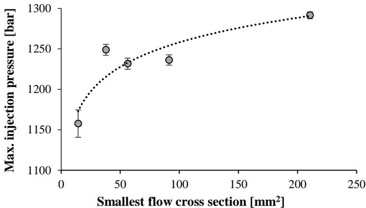
**Fig. 5.** Injection pressure as a function of the smallest flow cross section.
