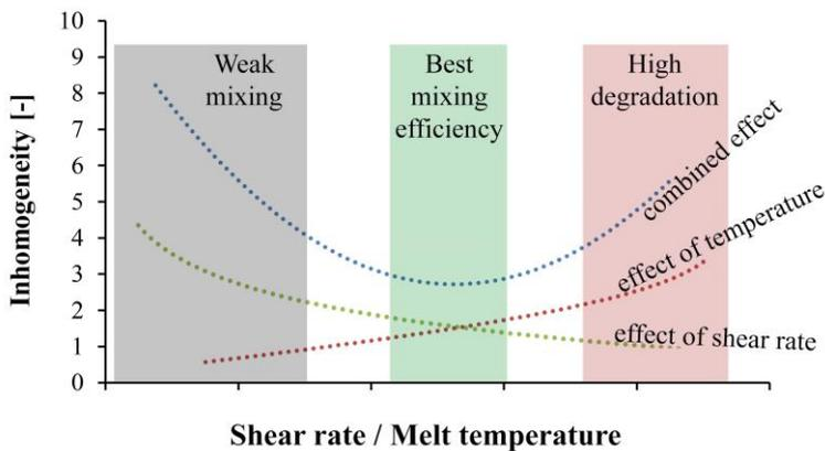
**Fig. 7.** The effects of the shearing action and melt temperature on color homogeneity.
