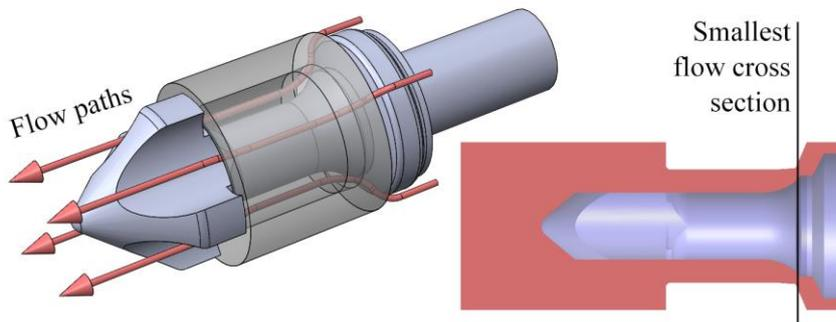
**Fig. 2.** Gap sizes of different dynamic mixer geometries
