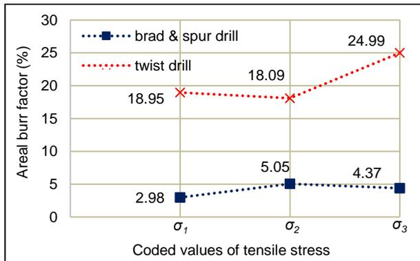
Fig. 5 Influence of tensile stress and tool geometry on areal burr factor
