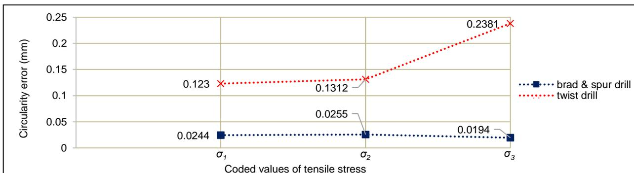
Fig. 7 Influence of tool geometry and tensile stress on circularity error
