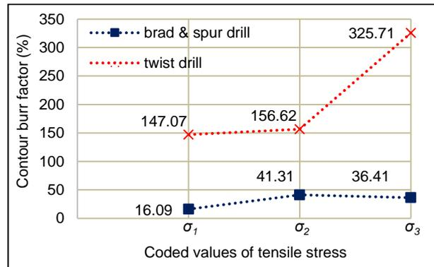
Fig. 6 Influence of tensile stress and tool geometry on contour burr factor
