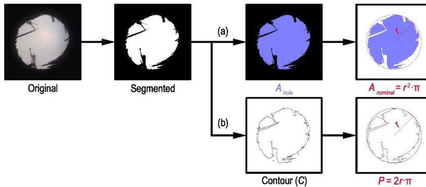
Fig. 4 Main steps of the digital image processing methods: (a) area-comparison based (b) contour-comparison based
