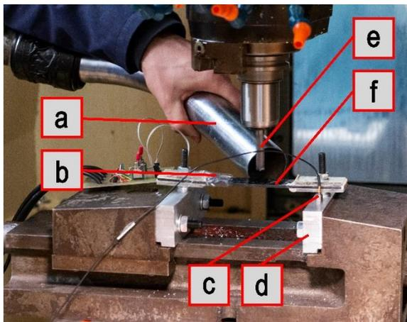
Fig. 2 Experimental setup: (a) vacuum cleaner (b) strain gauge (c) accelerometer (d) fixture jaw (e) drilling tool (f) UD-CFRP specimen
