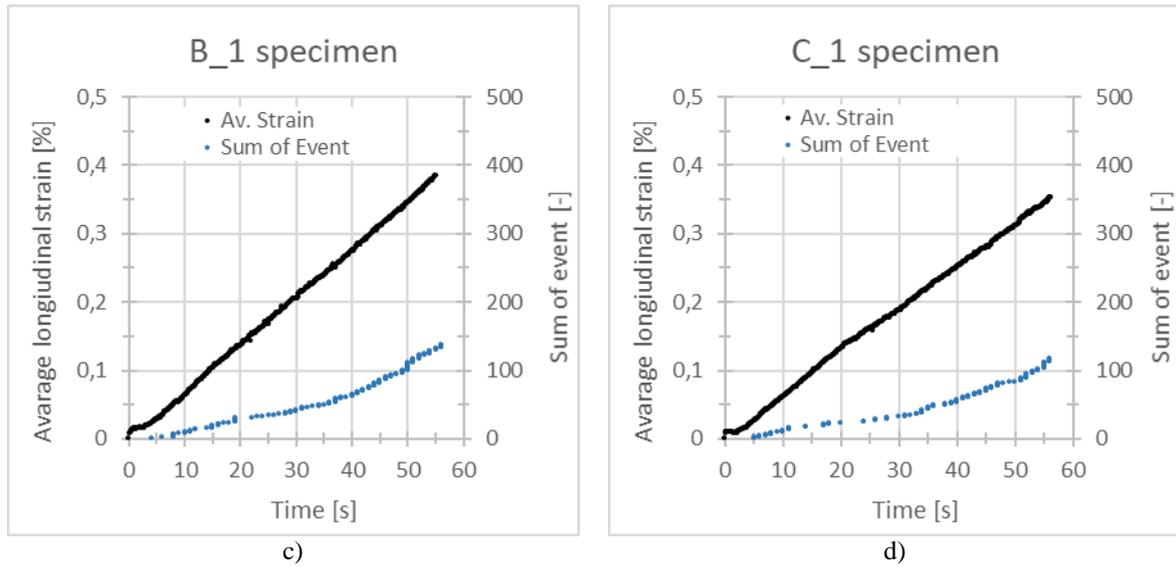
Figure 2: Elongation-time and sum of event-time correlation of different types of specimens: a) reference, b) A\_1, c) B\_1, d) C\_1 specimens.
