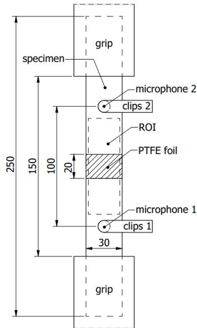
Figure 1: Geometry of specimen and location of measuring systems.
