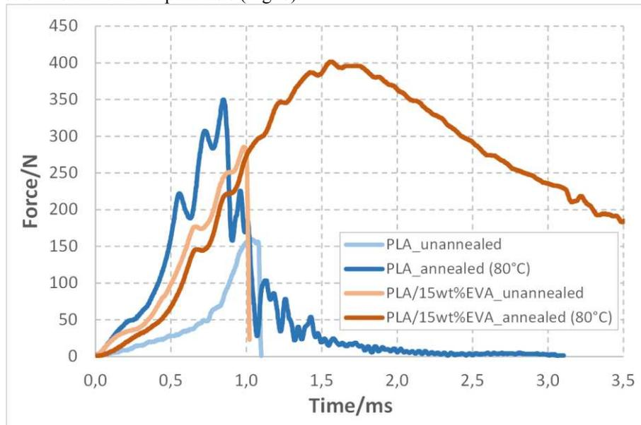
**Fig. 8 The fracturing process of unannealed PLA, annealed PLA (at  $80 \text{ }^\circ\text{C}$ ), unannealed PLA/15wt%EVA blend and annealed PLA/15wt%EVA blend (at  $80 \text{ }^\circ\text{C}$ ). The horizontal scale was only extended to 3.5 ms to show the differences between the curves of the various blends, even though the full fracture of the toughest blend only occurred after 7 ms**
