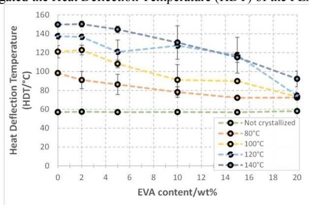
**Fig. 13 Heat deflection temperature of unannealed and annealed PLA/EVA blends**
