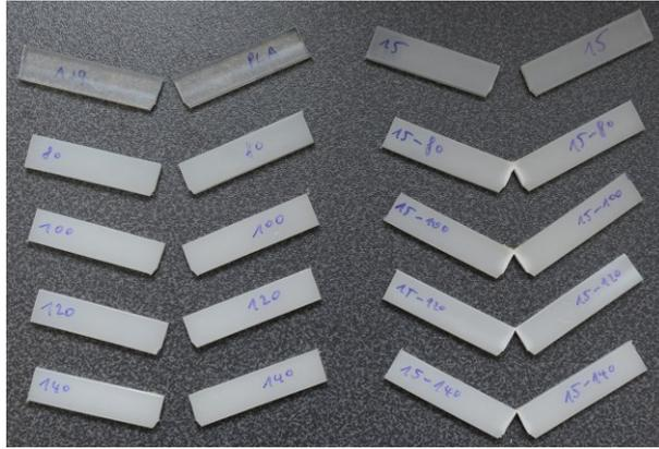
**Fig. 9** The Charpy tested fractured specimens. The specimens in the left column from top to bottom are unannealed pure PLA, and PLA annealed at 80 °C, 100 °C, 120 °C and 140 °C. The specimens in the right column from top to bottom are unannealed PLA/15wt%EVA blend, and annealed PLA/15wt%EVA blend at 80 °C, 100 °C, 120 °C and 140 °C
