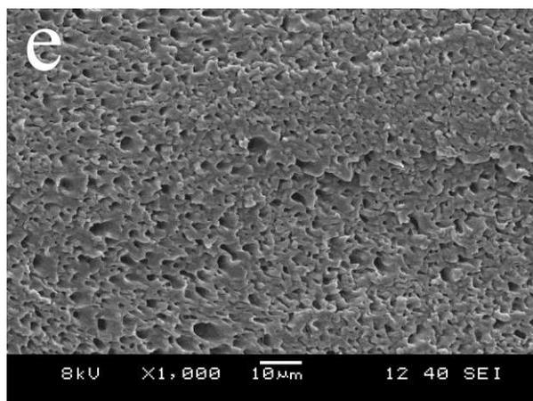
**Fig. 10 Charpy fracture surfaces of unannealed PLA (a), annealed PLA (b), unannealed PLA/15wt%EVA (c), annealed PLA/15wt%EVA (taken from the middle of the specimen) (d), and annealed PLA/15wt%EVA (taken from near the side of the specimen) (e)**
