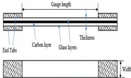
Figure 3. Specimen schematics.
