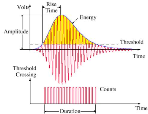
Figure 5. The definitions for acoustic-emission parameters [36].
