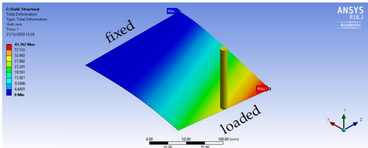
Figure 1 Finite element simulation of a cantilever bend-twist coupled composite under bending load. Total deformation plotted.
