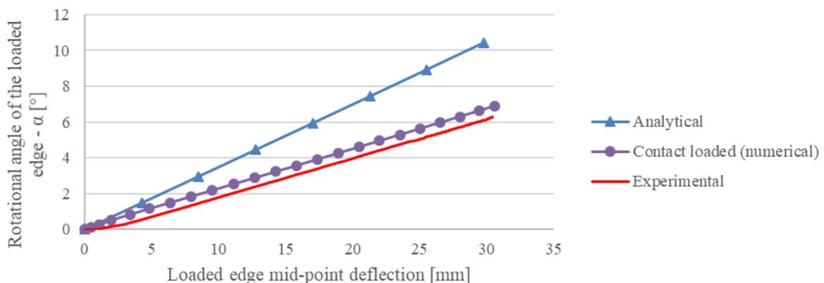
Figure 3 Analytical, numerical and experimental result comparison of the cantilever bending of a bend-twist composite plate. Rotational angle of the loaded edge as a function of the mid-point deflection of the loaded edge.
