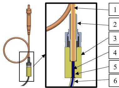
**Figure 3.** The connection of the fibre bundle in the cord-end terminal with the optical fibre in the standard subminiature assembly (SMA) connector (1: polymer optical fibre; 2: SMA connector; 3: the unique connector we developed; 4: reinforcing fibre bundle; 5: uninsulated cord-end terminal; 6: resin).
