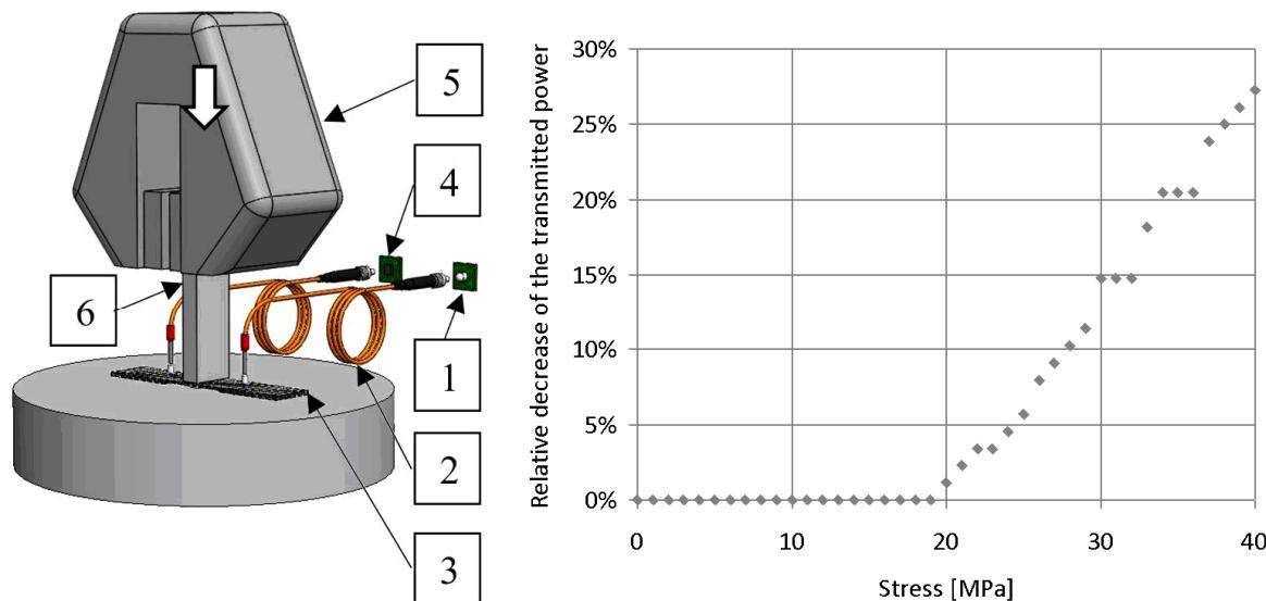
**Figure 4.** Compression measurement layout (1: light source, 2: signal transmitter (polymer optical fibre), 3: specimen, 4: photodiode, 5: clamp of the tensile tester, 6: compression fixture) and a typical plot.
