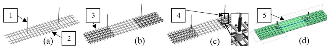
**Figure 1.** The steps of making a multifunctional composite specimen: (a) The selected fibre bundle (1) pulled out of the fabric (2) at both ends; (b) laying the second layer of reinforcement (3) on both sides; (c) putting the ends of the selected fibre bundle in cord-end terminals (4); and (d) the specimen soaked with resin (5).
