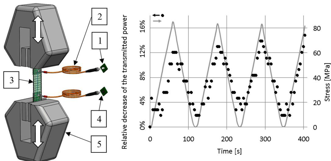
**Figure 6.** Cyclic tensile measurement layout (1: light source, 2: signal transmitter (polymer optical fibre), 3: specimen, 4: photodiode, 5: clamp of the tensile machine) and a typical plot.
