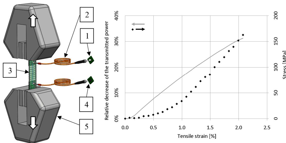
**Figure 5.** Tensile measurement layout (1: light source, 2: signal transmitter (polymer optical fibre), 3: specimen, 4: photodiode, 5: clamp of the tensile machine) and a typical plot.
