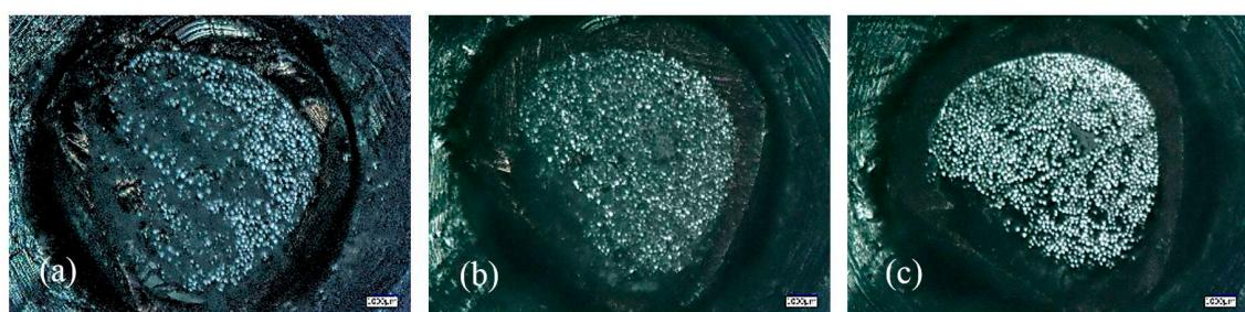
**Figure 2.** Microscope images of (a) a fibre bundle held together after cutting, and (b) 30- $\mu\text{m}$  (c) and 0.2- $\mu\text{m}$  fineness polishing.
