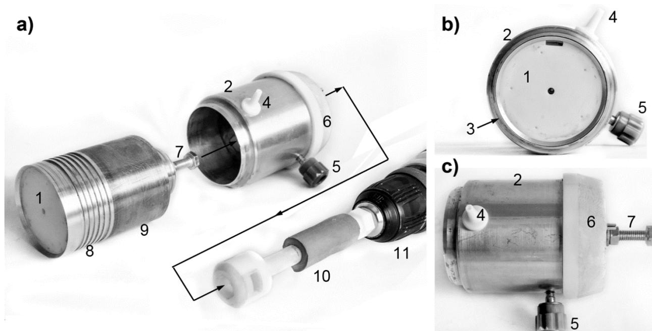
Figure 2. The spinneret in a) exploded, b) top and c) side views. 1: rotor, 2: stator, 3: orifice, 4: solution inlet, 5: high voltage connector, 6: base, 7: hexagonal drive connection, 8: solution take-up thread, 9: sliding bearing, 10: flexible plastic/rubber shaft, 11: chuck
