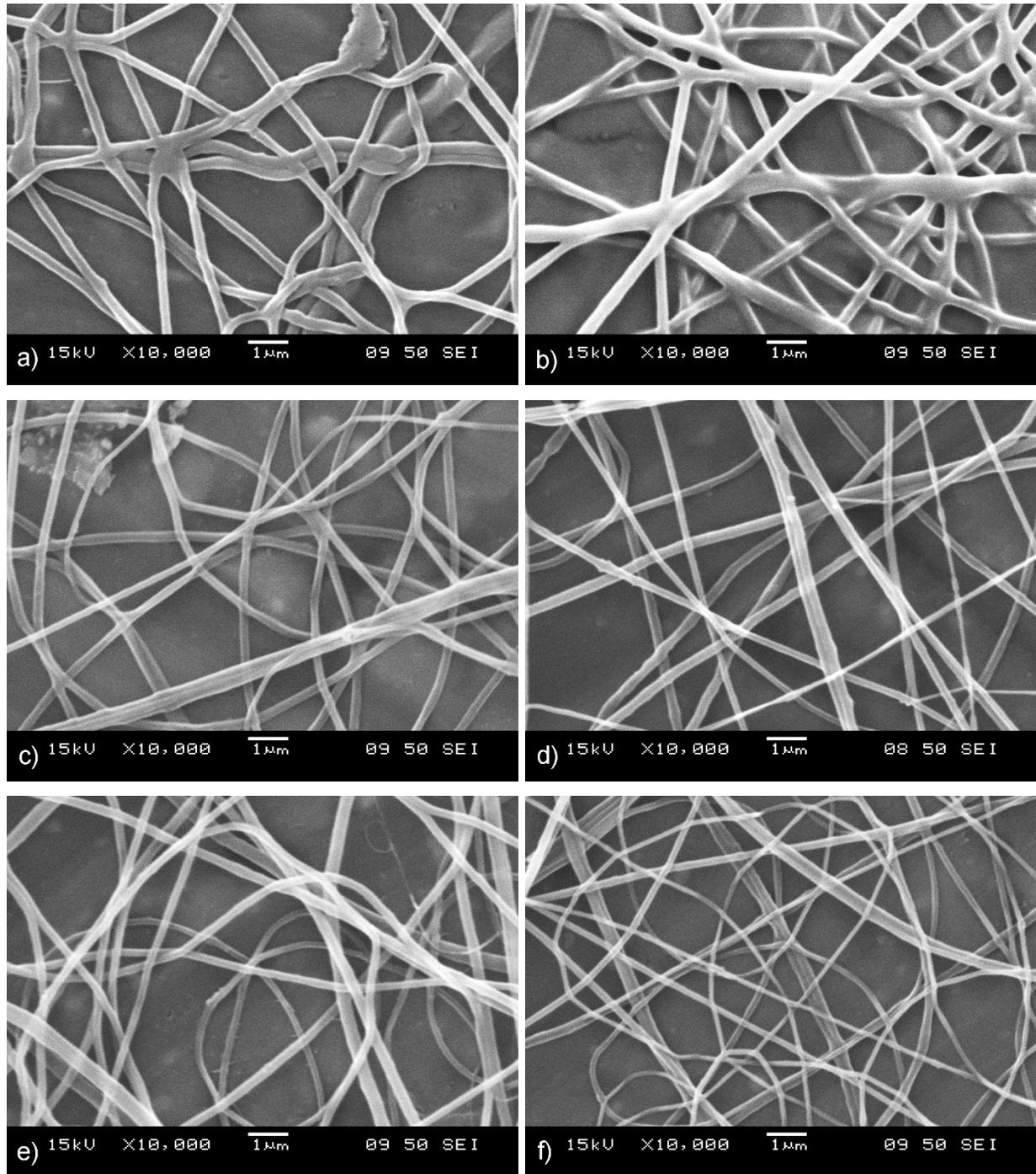
Figure 6. Fibers collected at different rotation speeds, a) 0 rpm, b) 75 rpm, c) 150 rpm, d) 300 rpm, e) 500 rpm, f)750 rpm
